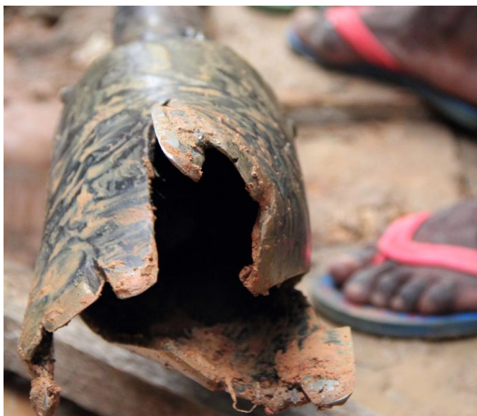
Figure 12: Jetting Cutting Shoe used in Lagos, Nigeria (Source: Kerstin Danert)
