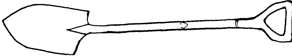
Name: SHOVEL Local Name: Pala Description and Use: A tool with a broad scoop and long handle, used for lifting and moving loose materials.
