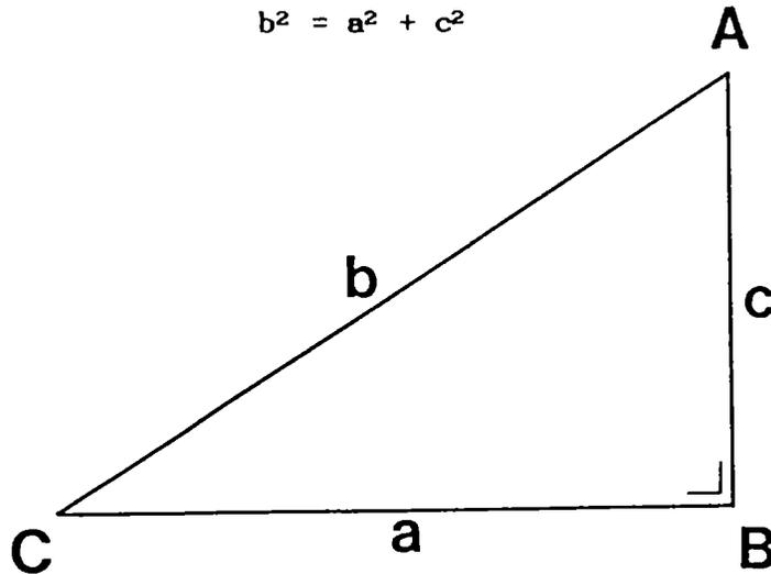
For most triangles the arithmetic, whilst simple, produces lines with dimensions that are difficult to construct accurately on site. One triangle, however, is relatively straightforward : a right-angled triangle can have a hypotenuse of 5 and the other two sides lengths of 3 and 4, respectively, which makes it very simple to construct on site a triangle with an internal angle of 90°.
