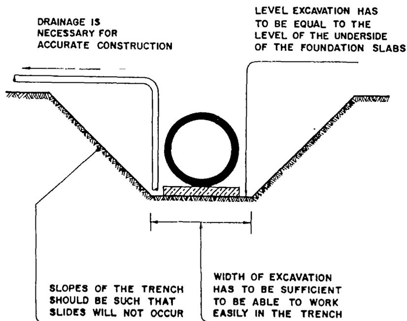
*Fig. 1. Excavation requirements for the laying of pipes*
