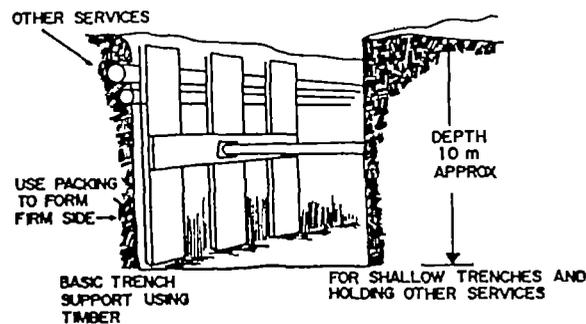
*Fig. 2. Supporting trench sides*
