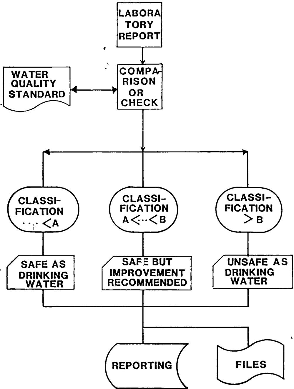
Fig. 1. Water quality monitoring; flow chart.
