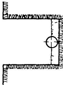
2. TAMP SOIL UNDER PIPES AND BETWEEN PIPELINE AND TRENCH WALL AT BOTH SIDES. WATER TAMPING MAY BE USED WHERE DRAINAGE IS GOOD.
