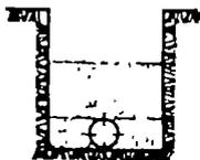
5. Backfilling by hand until 20 cm over the pipe. Tamp each 10 cm layer.
