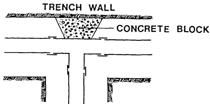
Fig. 4. Thrust block at T-junction.
