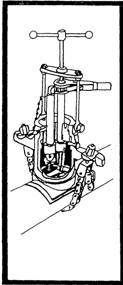
*Fig. 4. Equipment for tapping A.C./steel pipes under pressure.*
