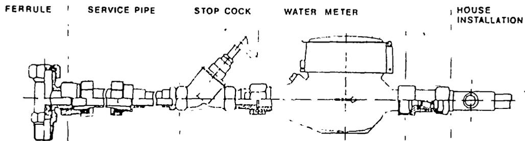
Fig. 1. Typical service connection assembly
