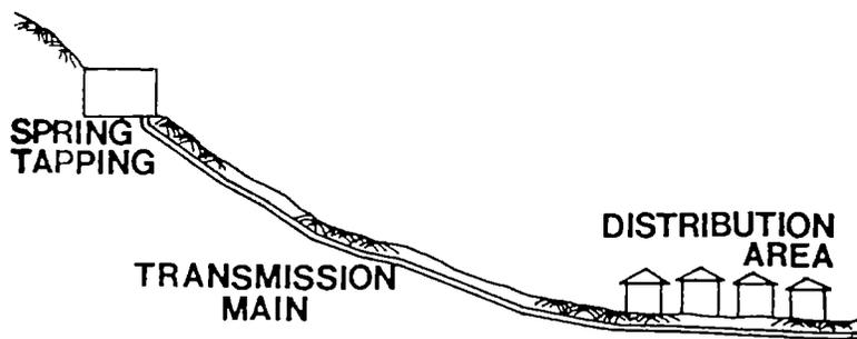
*Fig. 2. Gravity flow system.*
