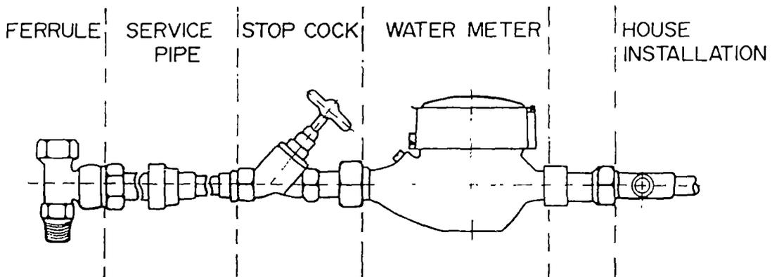
Fig. 1. Typical service connection assembly.
