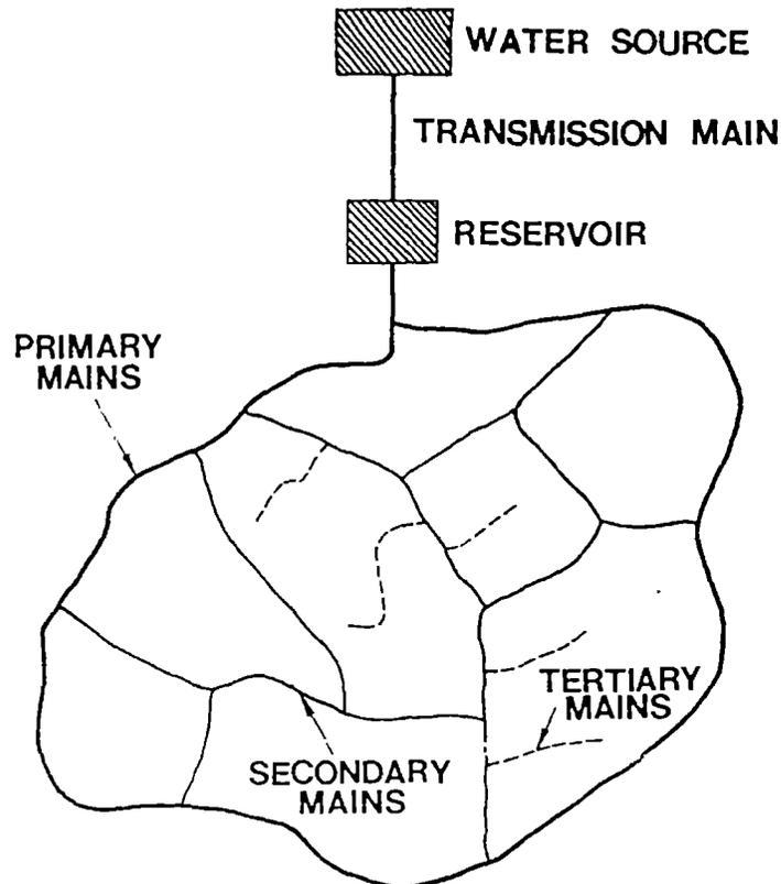
*Fig. 7. Schematical lay-out of distribution system.*
