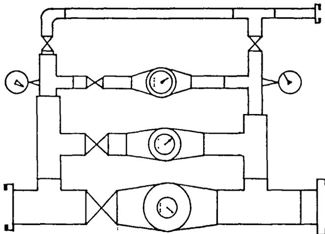
Fig. 2. Portable waste meter assembly
