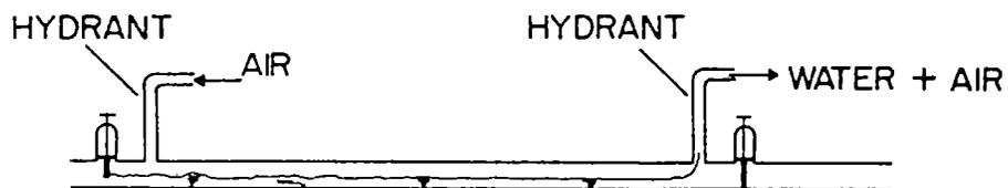
*Fig. 1. Air/water flushing.*
