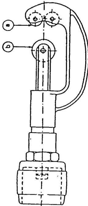
PIPE CUTTER (SMALL-DIAMETER PIPE)
