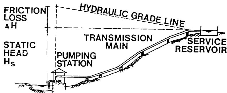
*Fig. 3. Pumped system.*
