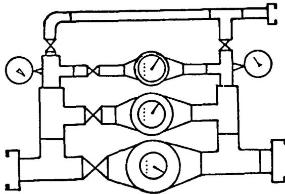
*Fig. 2. Portable waste meter*
