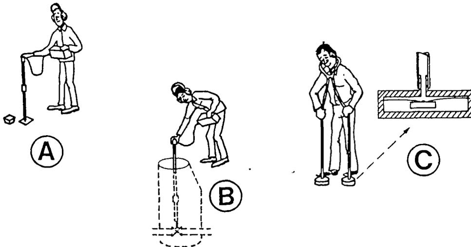
*Fig. 4. Leak sounding methods*
