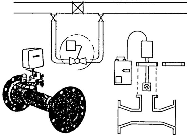
Fig. 3. Typical permanent waste meter
