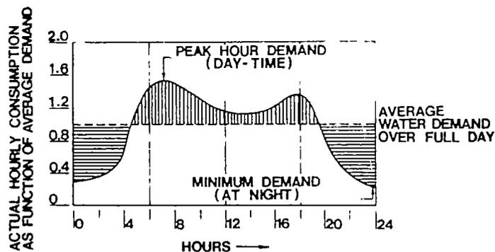
*Fig. 4. Daily fluctuation of water consumption.*
