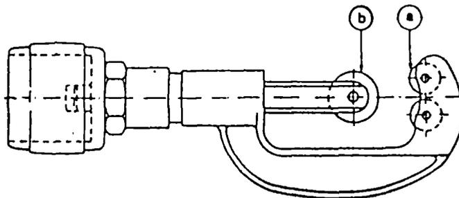
Fig. 2. Pipe cutter (for small-diameter pipe)
