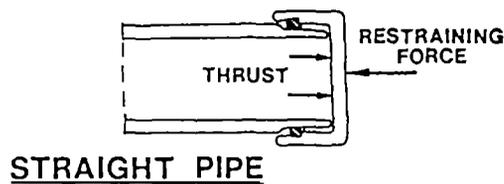
Fig. 2. Forces acting on end of pipe.
