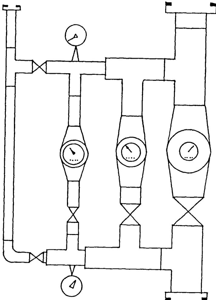
TYPICAL PORTABLE WASTE METER ASSEMBLY
