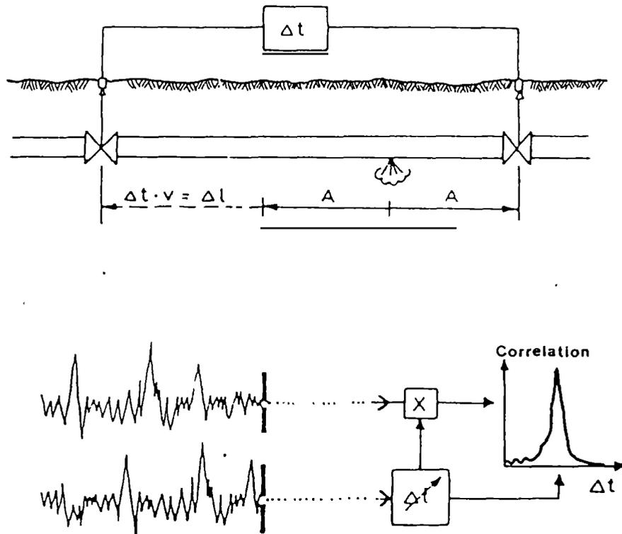
*Fig. 4. Principle of the correlation process.*
