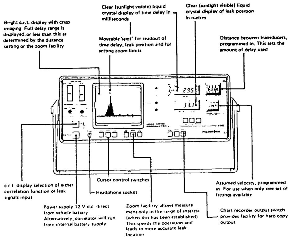
Fig. 5. Leak-noise correlator.
