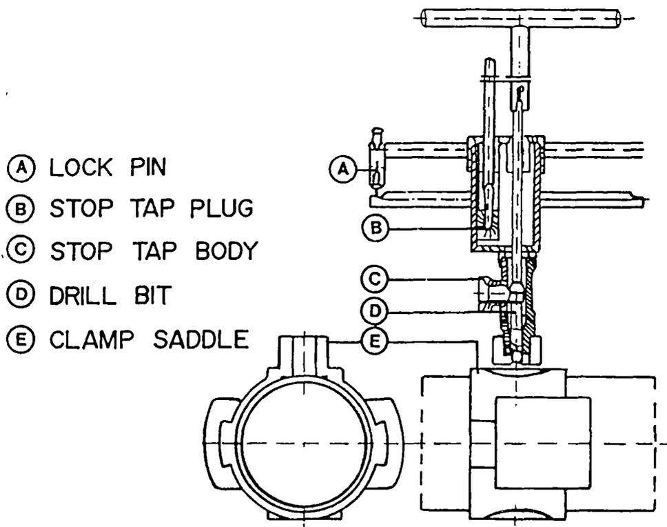
Fig. 5. Equipment for tapping uPVC pipe under pressure.
