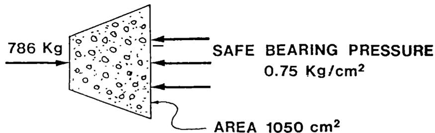
*Fig. 5. Forces acting on thrust block.*
