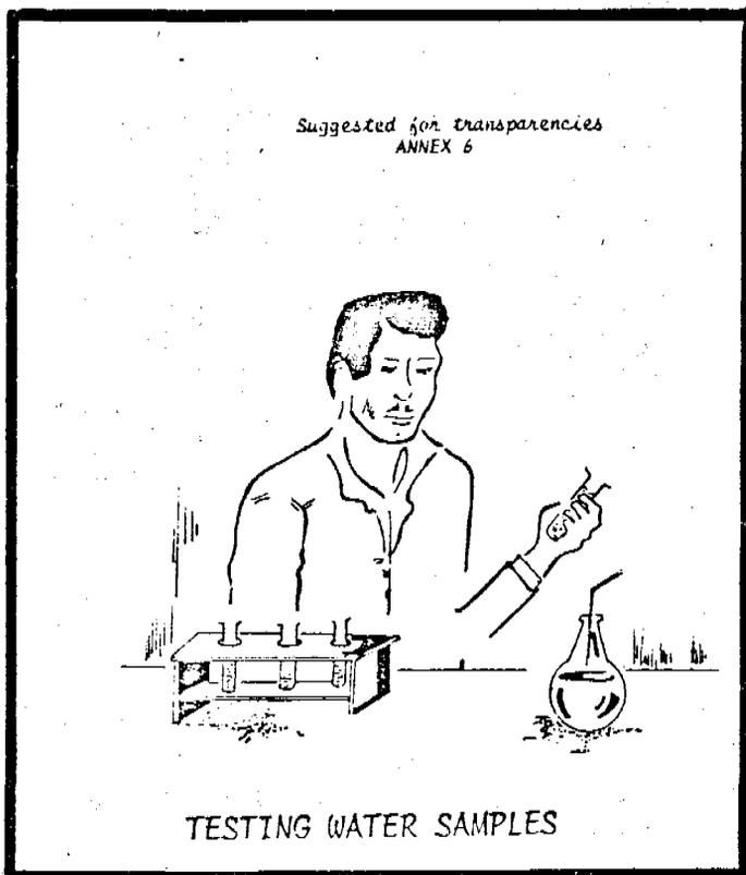
The treatment plant operator tests samples of water frequently in order to determine what treatment is necessary. He knows, for example, that if too many chlorides are present, the water will taste salty and may corrode the pipes. He knows that if the water contains too much iron, it may stain clothing and plumbing fixtures and spoil the taste of beverages.
