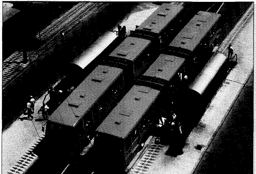
Figure 2 (below) Two of the special bi-articulated buses with a carrying capacity of 270 passengers at a tube station
