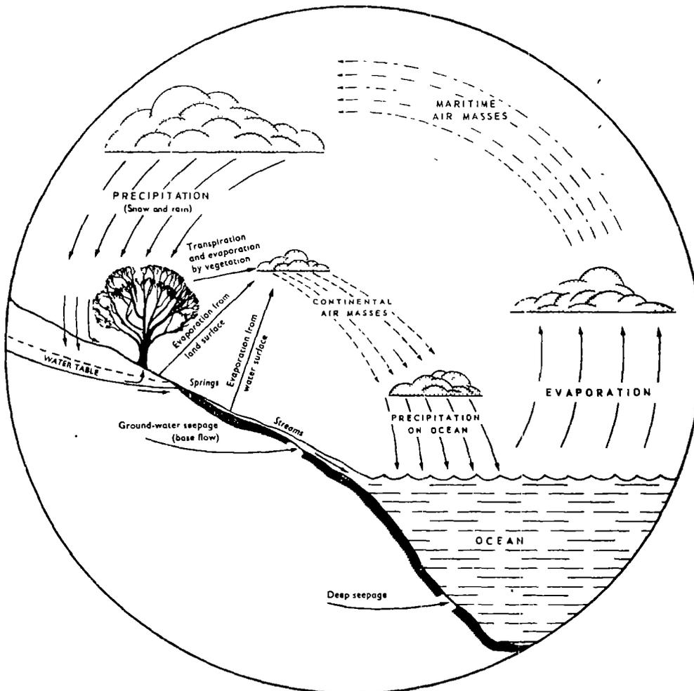
Figure 4-1. Schematic representation of the hydrological cycle./6/
