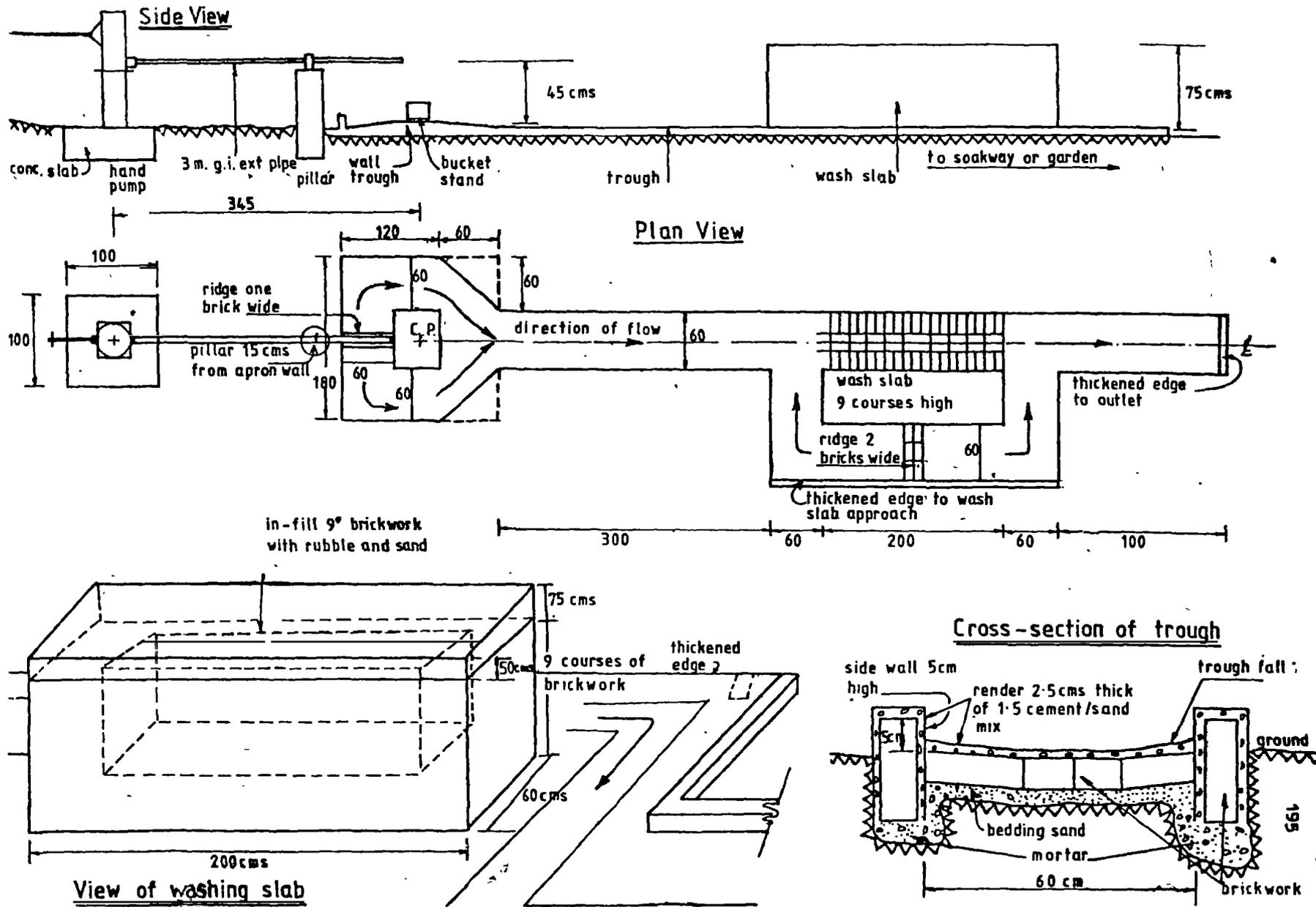
Figure 11-8. Typical hand pump installation in Malawi./17/
