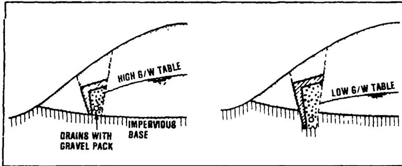
Figure 10-2. Tapping of a gravity spring./18/
