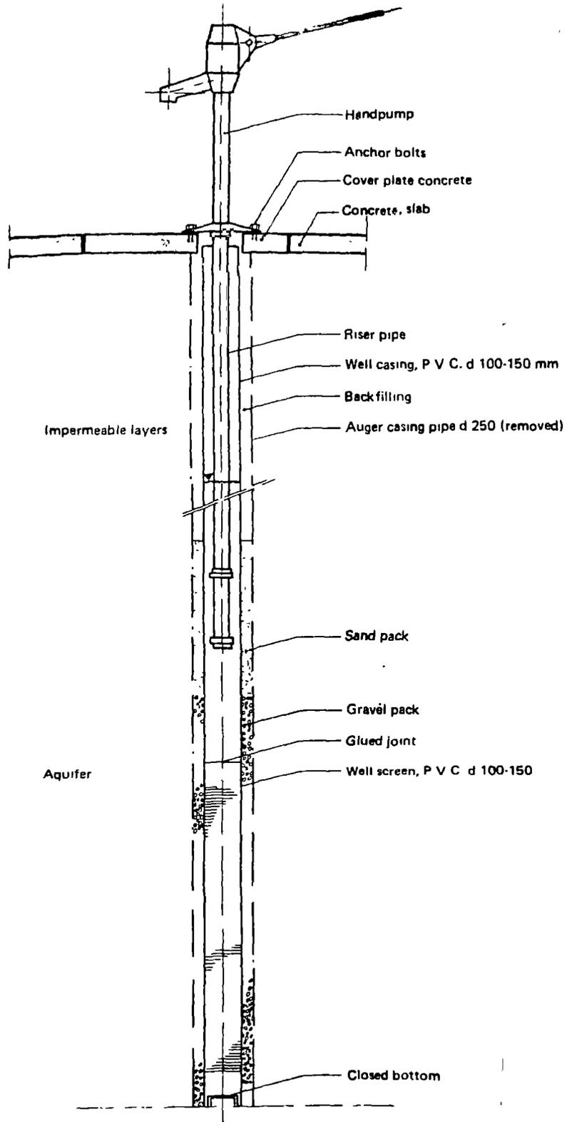
Figure 8-13. Hand auger well./29/
