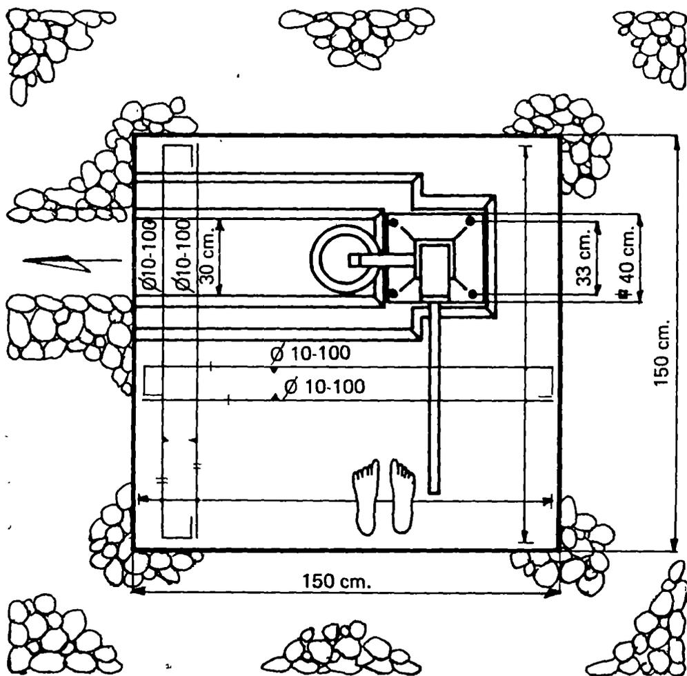
Figure 9-10. Example of a superstructure for a SWN hand pump consisting of a reinforced concrete slab, a pump base with anchor bolts and a gutter.
