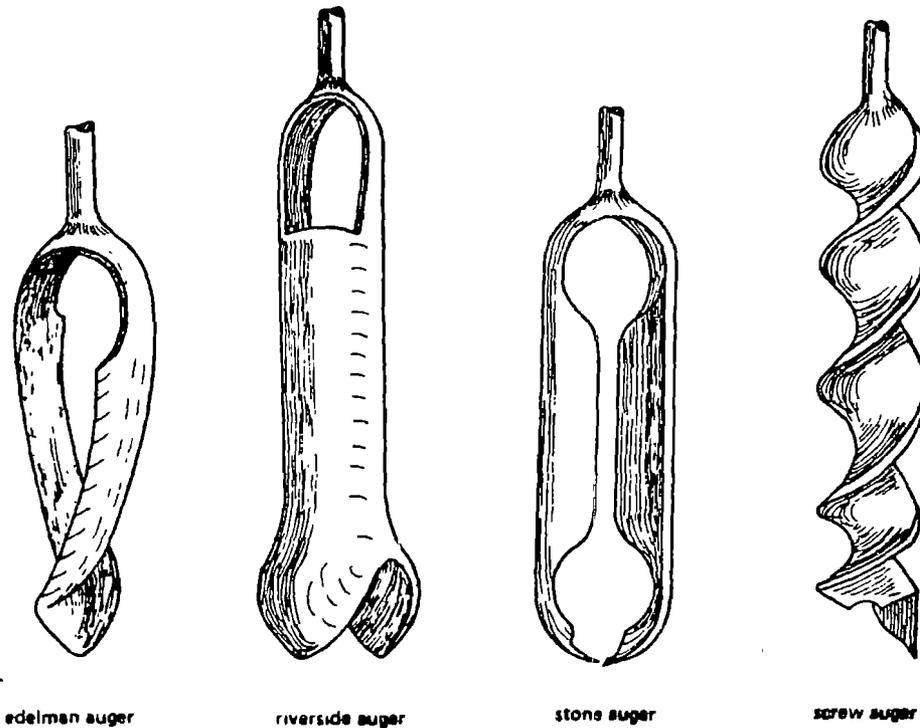
Figure 7-11. Hand auger equipment./ B/
