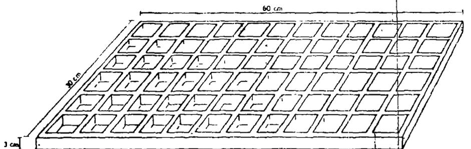
Figure 7-13. Box for rock/soil samples. /13/
