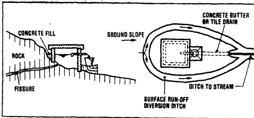
Figure 10-4a. Fissure spring of small capacity./18/
