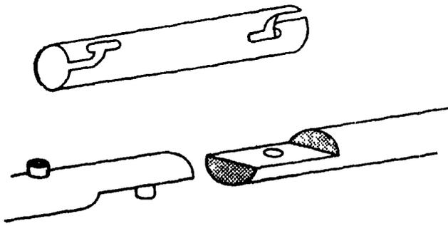
**Coupling system for drilling rods.**
