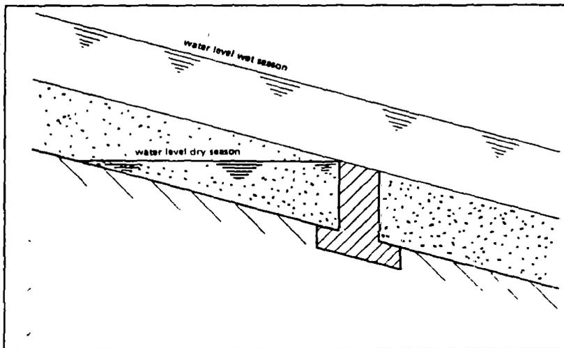
Figure 10-6. Small clay dam in a sandy riverbed./ 8 /
