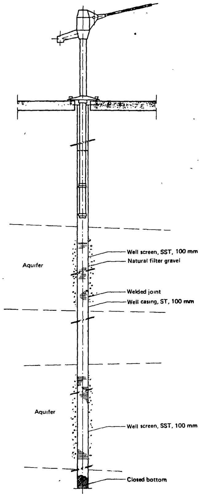
Figure 8-10. Machine auger well./29 /
