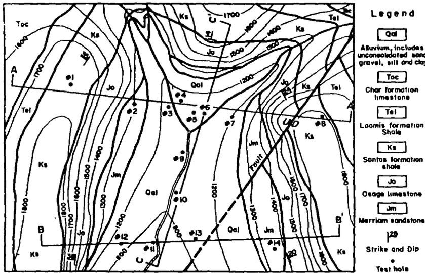
Figure 7-1. Example of a geological map showing test hole locations./16/
