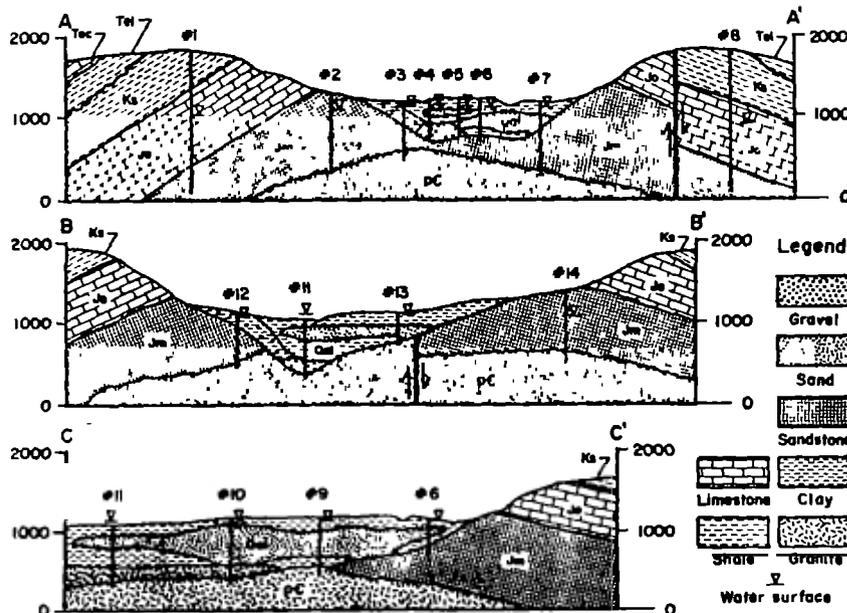
Figure 7-2. Geologic cross-section from the map of figure 7-1./16/
