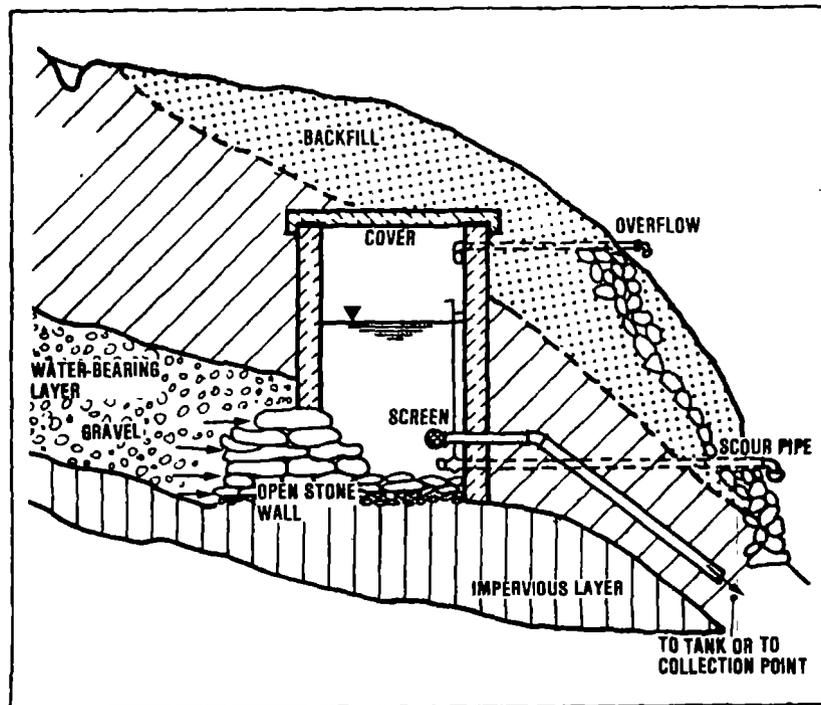
Figure 10-3. Spring water storage chamber ('spring box')./18/
