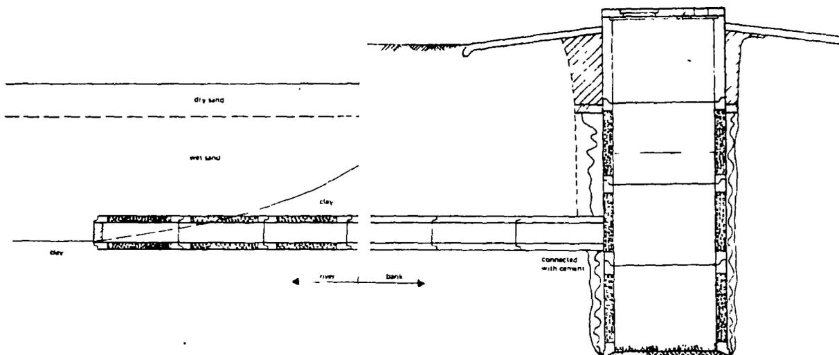
Figure 10-7. River well with small concrete rings in the trench./ 8 /
