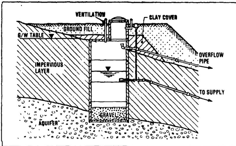
Figure 10-4b. Fissure spring of large capacity./18/
