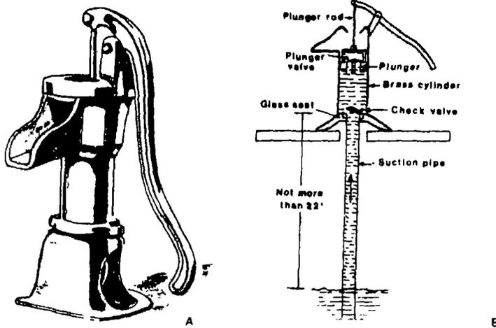
Figure 9-1a. Typical shallow well lift pump./22/
