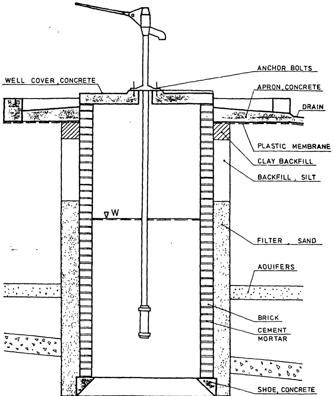
Figure 11-7. Shallow well lined with bricks./20/
