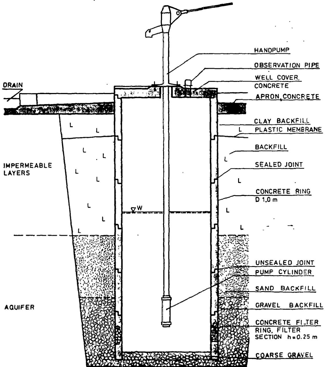
Figure 8-5. Machine excavated water well./29/
