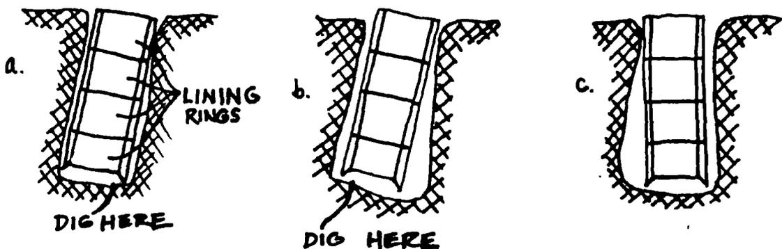
Figure 8-9. Straightening well rings in loose soils./5/
