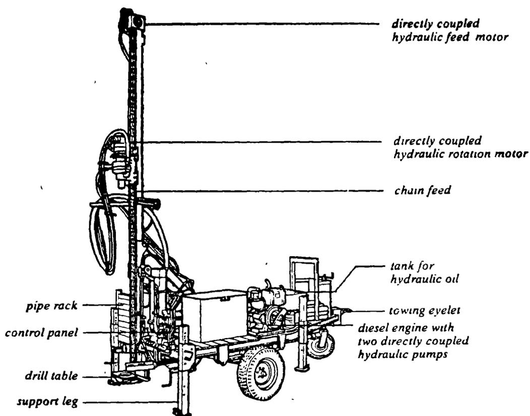
Figure 8-11. Water well drilling machine.
