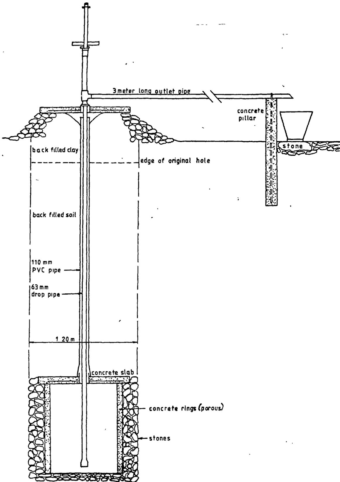
Figure 11-6. Recommended dug well construction./17/
