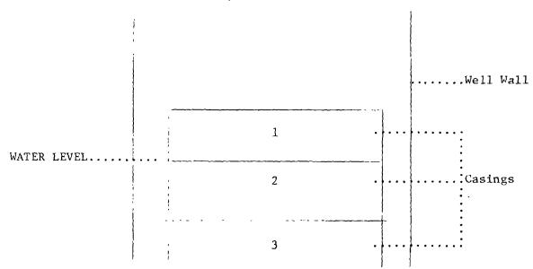
Although there are holes in the sides of these casings, there is no gravel between the casing and the well wall; thus, sand rushes into the water. Even if gravel is used, it will not sink into the sand as the heavy casings will, but will be halted by the sand.
