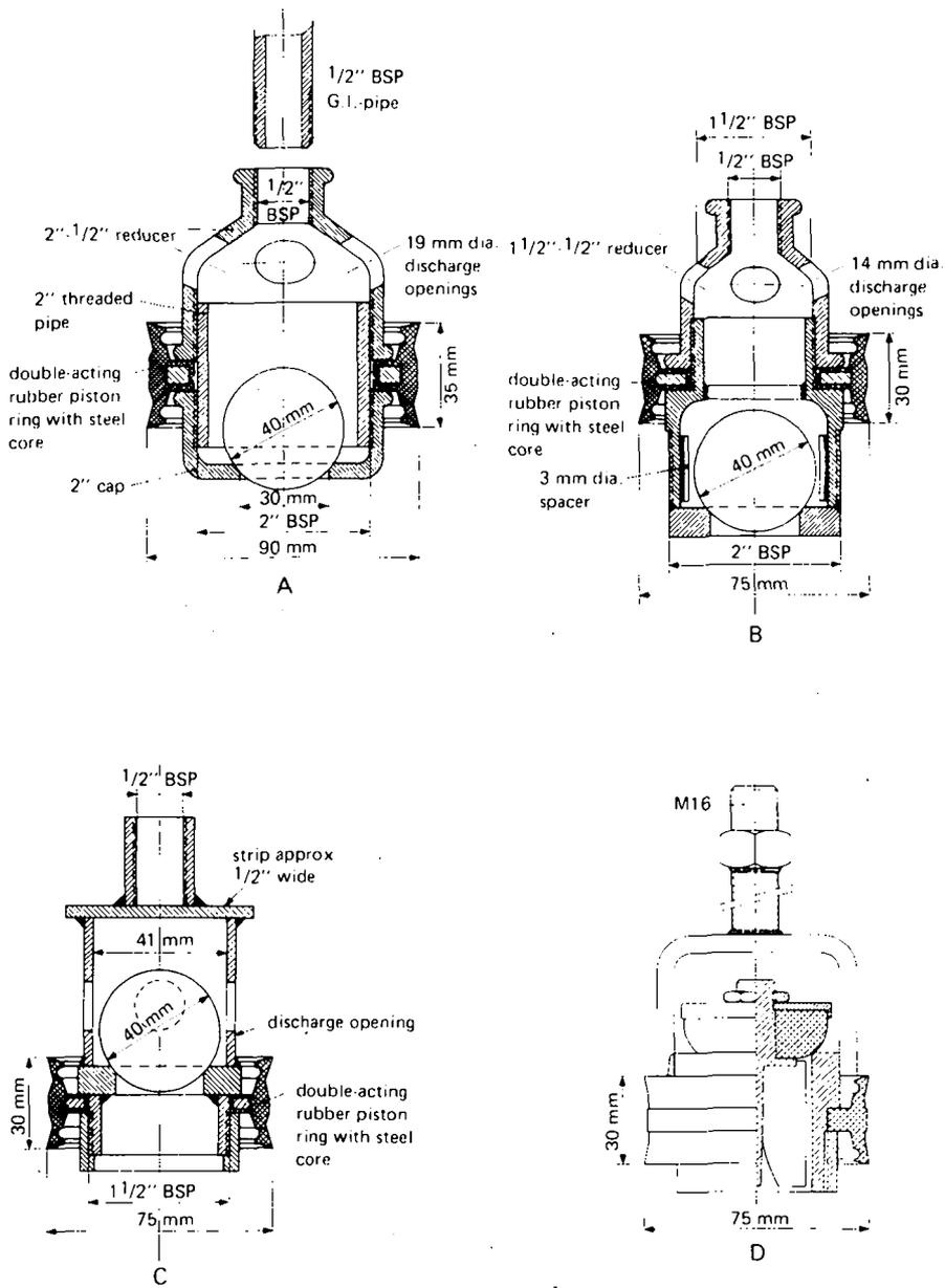
Fig. 35. Development of pump piston
