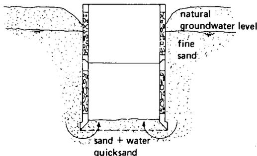
Experience has taught that one should not try to construct a well in a layer of fine or medium sand that is more than about 3 metres thick, since at this depth it is no longer possible to continue digging against the sand entering from underneath, which means the rings cannot sink any farther.
