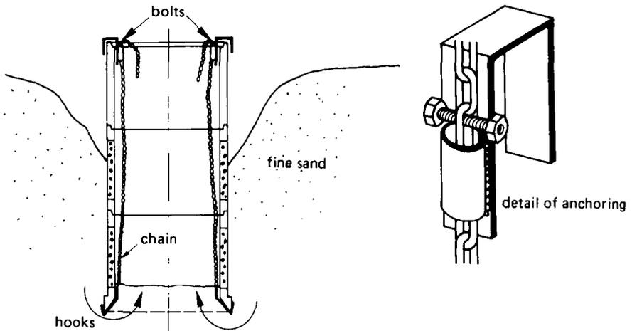
Fig. 19. Preventing uneven setting of well rings
