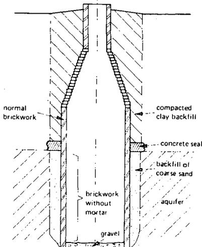
Fig. 25. Well with in-situ brick lining.
