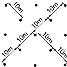
Fig. 10. Drilling pattern in wet places
