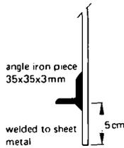
Fig. 24. Auxiliary angle iron supports.
