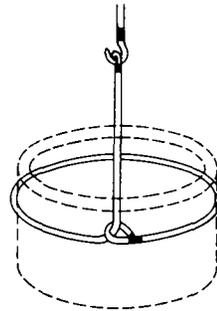
Fig. 30. Sling for turning over a concrete ring
