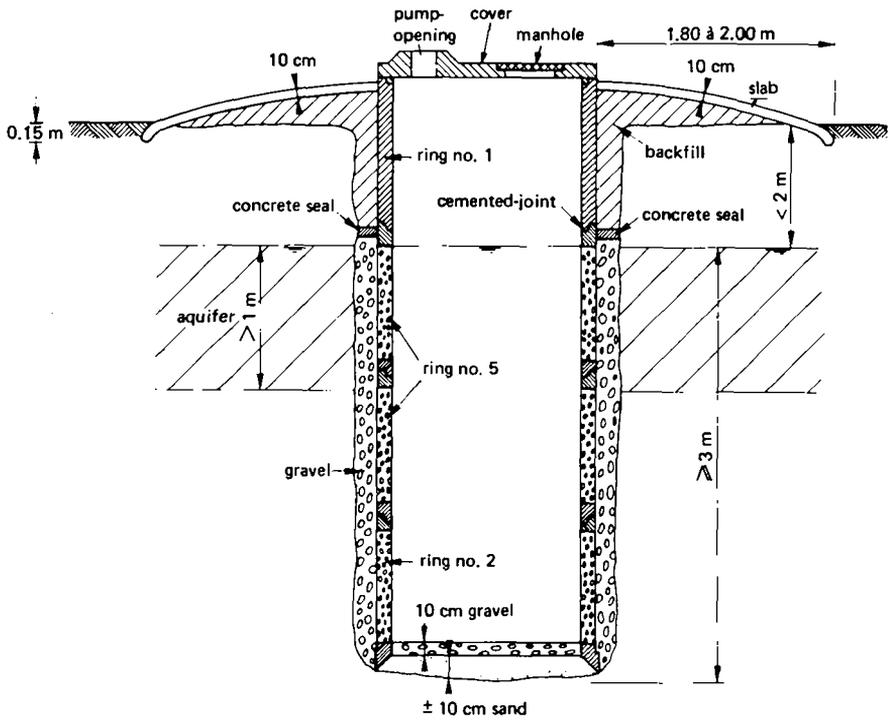
Fig. 17. Standard well (type A)
