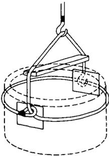
Fig. 29. Sling for lifting a concrete ring horizontally
