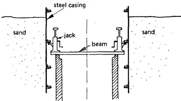
Fig. 20. Removing steel casing with jacks.
