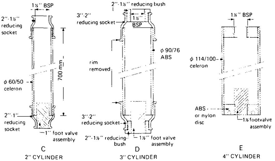
opening with  $1\frac{1}{2}$ " BSP thread (fig. 33B). The rising main is screwed into the upper flange, while the foot-valve assembly fits in the bottom flange as shown in fig. 34D.
