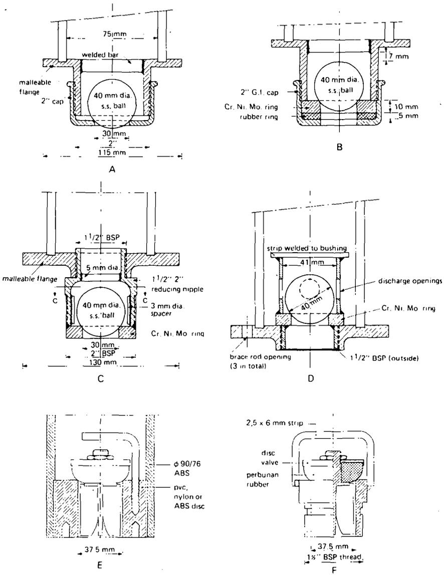
Fig. 34. Alternative constructions of foot-valve assembly
