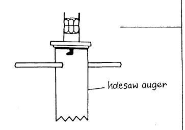
Use Holesaw Auger for drilling in decomposed rock! Attach as for standard Auger. See step 7.
