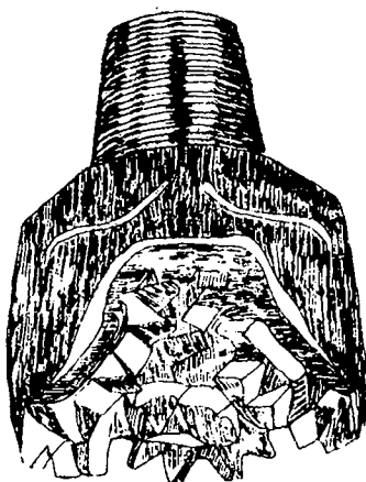
Fig. 4.11. Three Cone Rock Roller Bit for Soft Formations with Conventional Mud Discharge Ports
