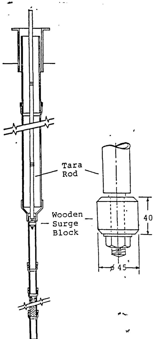
Fig. 4 : Using a Wooden Surge Plunger with Tara Rods
