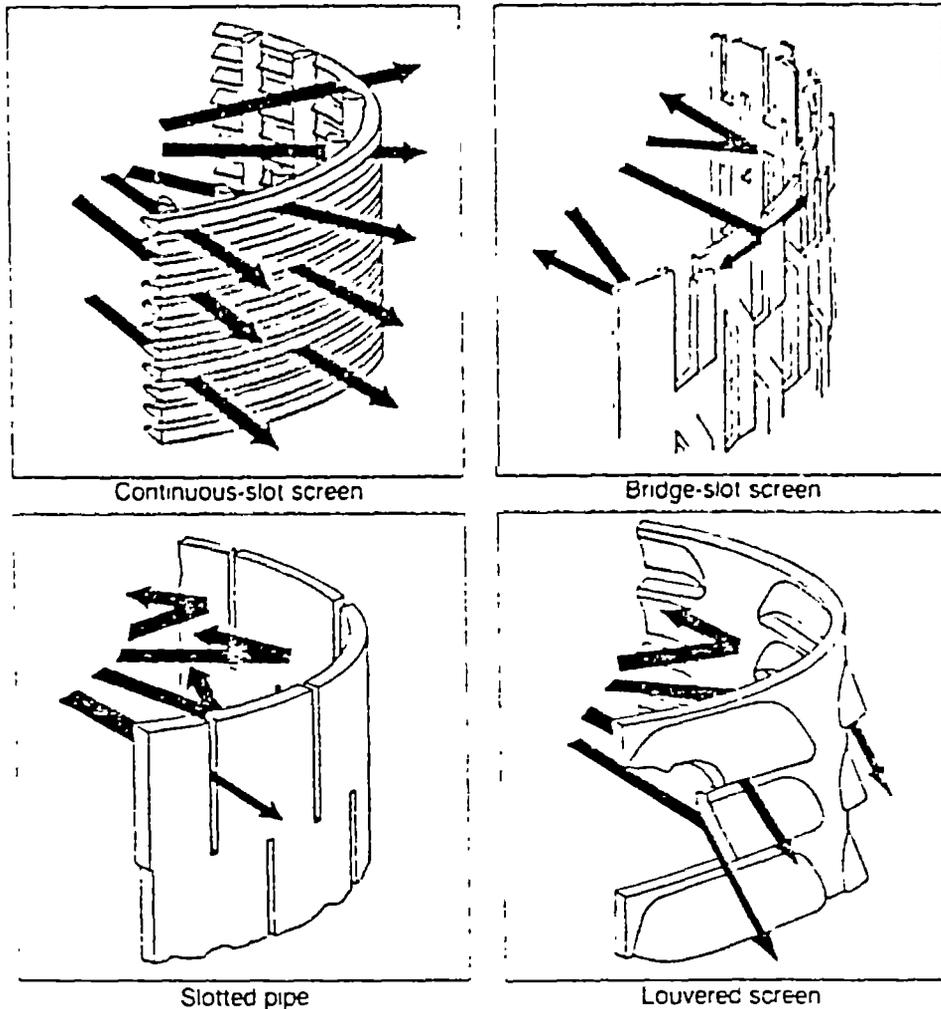
Figure 15.15. The open area of the screen and the configuration of the slot openings are important factors controlling the effectiveness of development procedures using water jetting.
