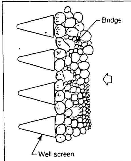
Figure 15.4. During development by overpumping, sand grains can bridge openings because flow occurs in only one direction. Once the well is placed into service, agitation by normal pump cycling can break down the bridges, causing sand pumping.
