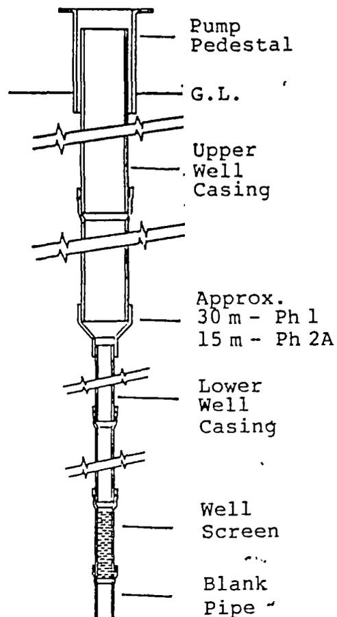
Fig.2 : General Casing Configuration
