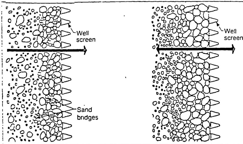
Figure 15.5. Effective development action requires movement of water in both directions through screen openings. Reversing flow helps break down bridging of particles. Movement in only one direction, as when pumping from the well, does not produce the proper development effect.
