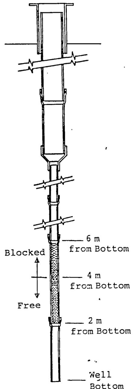
Fig. 3 : Free & Blocked Casing
