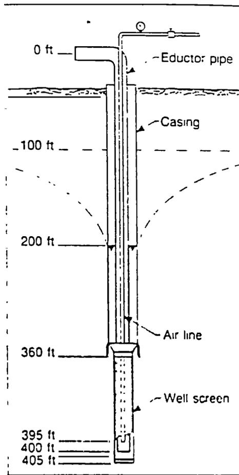
Figure 15.14. Determining the design of an air-lift system for a specific well.
