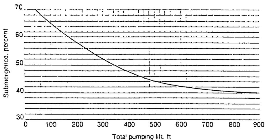
Figure 15.13. Approximate percent pumping submergence for optimum air-lift efficiency. In general, development proceeds most efficiently when the discharge is maximized. Therefore, the submergence should always be as great as possible within practical limits. (Ingersoll-Rand, 1971)
