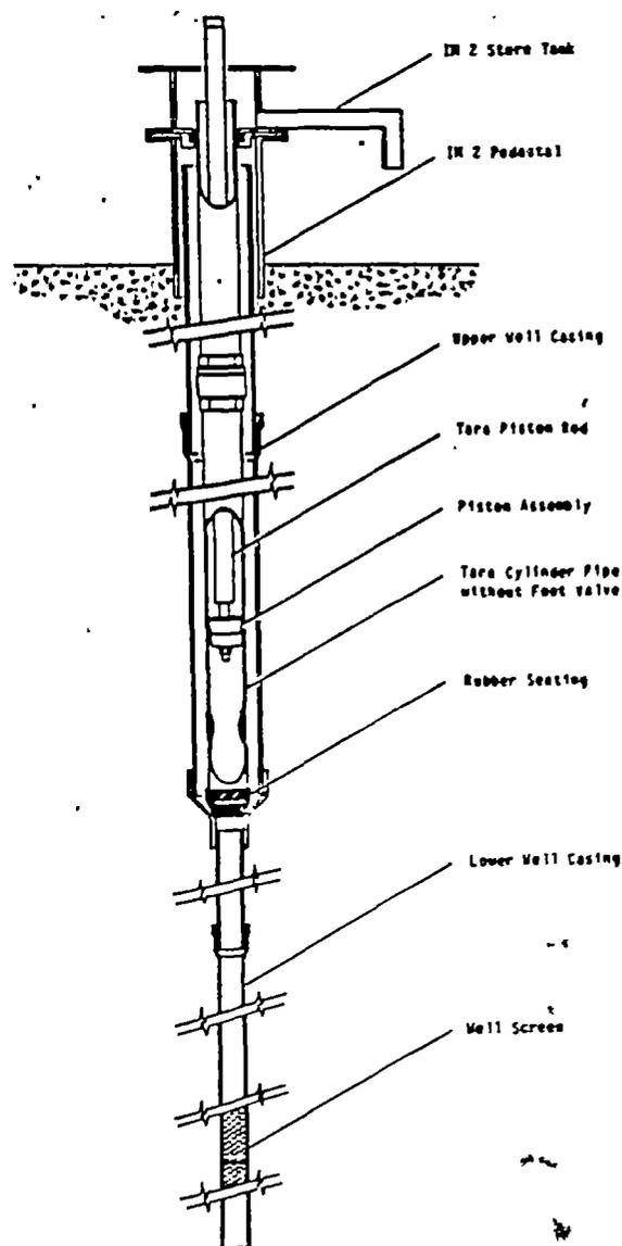
Fig. 8 : Manual Well Cleaning & Over pumping using the Tara DA Pump components
