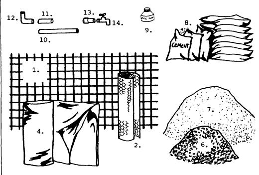
Note: for larger tanks you will need more materials; for an elevated tank you will need 15 concrete blocks and approximately 10 x 40kg 88lb bags of gravel/aggregate to raise the tank by one layer of blocks
