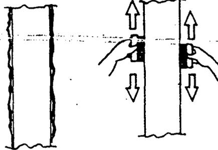
Scraping out excessive mortar build-up. This also improves adhesion of finishing coat.
