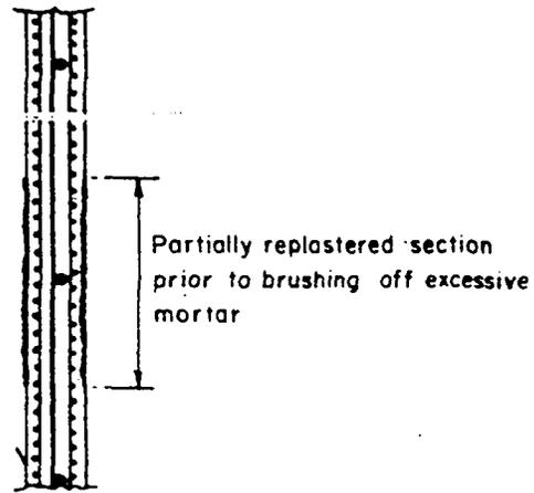
(b) Repair partially complete
