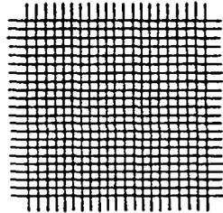
2 Layers of mesh perfectly mis-aligned (correct practice)
