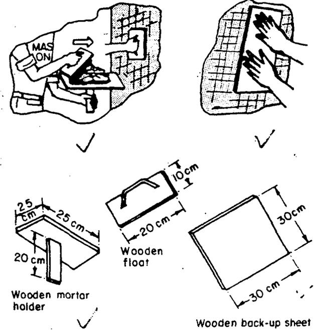
(b) Plastering technique and simple equipments that make plastering an easy task. Mason impregnates mortar from the inside of the tank while the helper holds a back-up sheet on the outside
