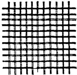
2 Layers of mesh not mis-aligned (incorrect practice)
