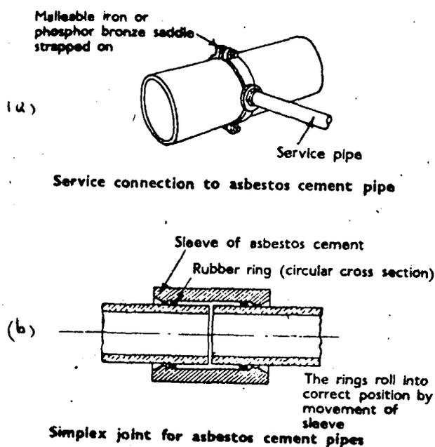
Fig 7 (a) Service Joint (b) Simplex joint for A-C Pipe (10)
