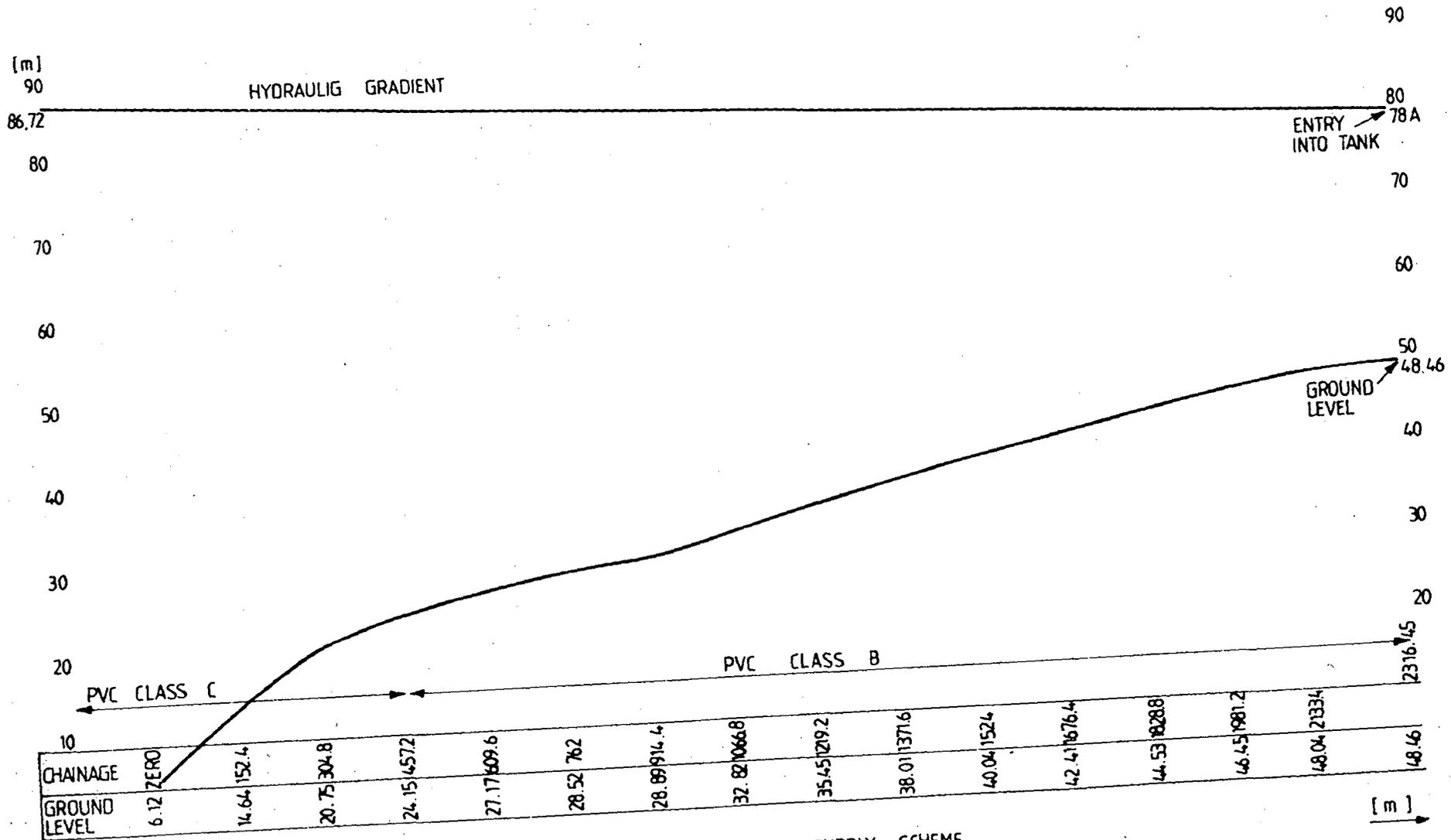
FIG: 14 PROFILE FOR MANSA WATER SUPPLY SCHEME
