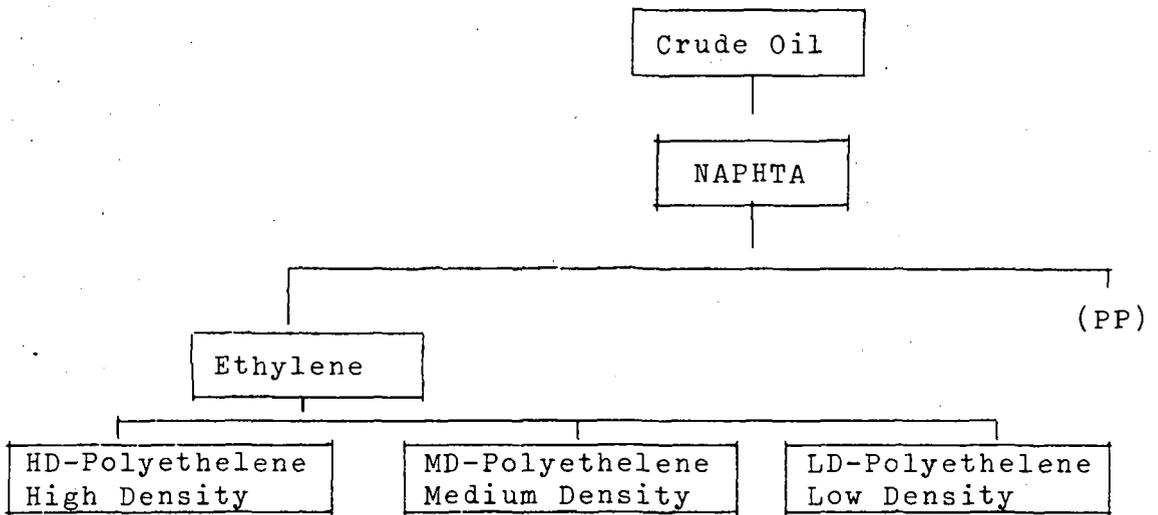
HD-Polyethelene (HDPE) is produced through a low pressure process. MD-Polyethelene (MDPE) and LD-Polyethelene (LDPE) are obtained through a relatively high pressure method in which the quality of the product depends on the pressure. The raw material also plays an important role. In the HDPE the crystallinity of the raw material is more than that of the LDPE and this accounts for the hardness in the former.
