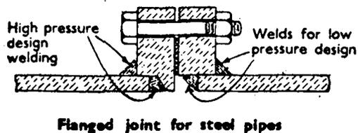
Pipes may also be bevel-ended for bult welding. The common flanged joint is also shown in Fig.8.
