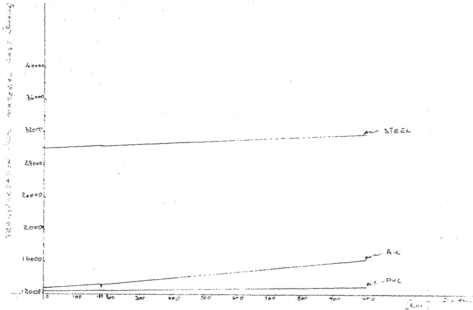
Fig. 18. Transportation plus material costs vs distance
