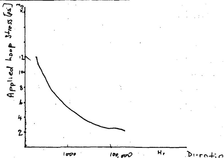
This means that the safety factor should be established for long hours of stress application. Using, for example 100,000 hour stress application, the design stress upon which pressure rating is based is then defined by dividing the 'hoop' stress established on the stress regression curve at 100,000 hour by a chosen safety factor.
