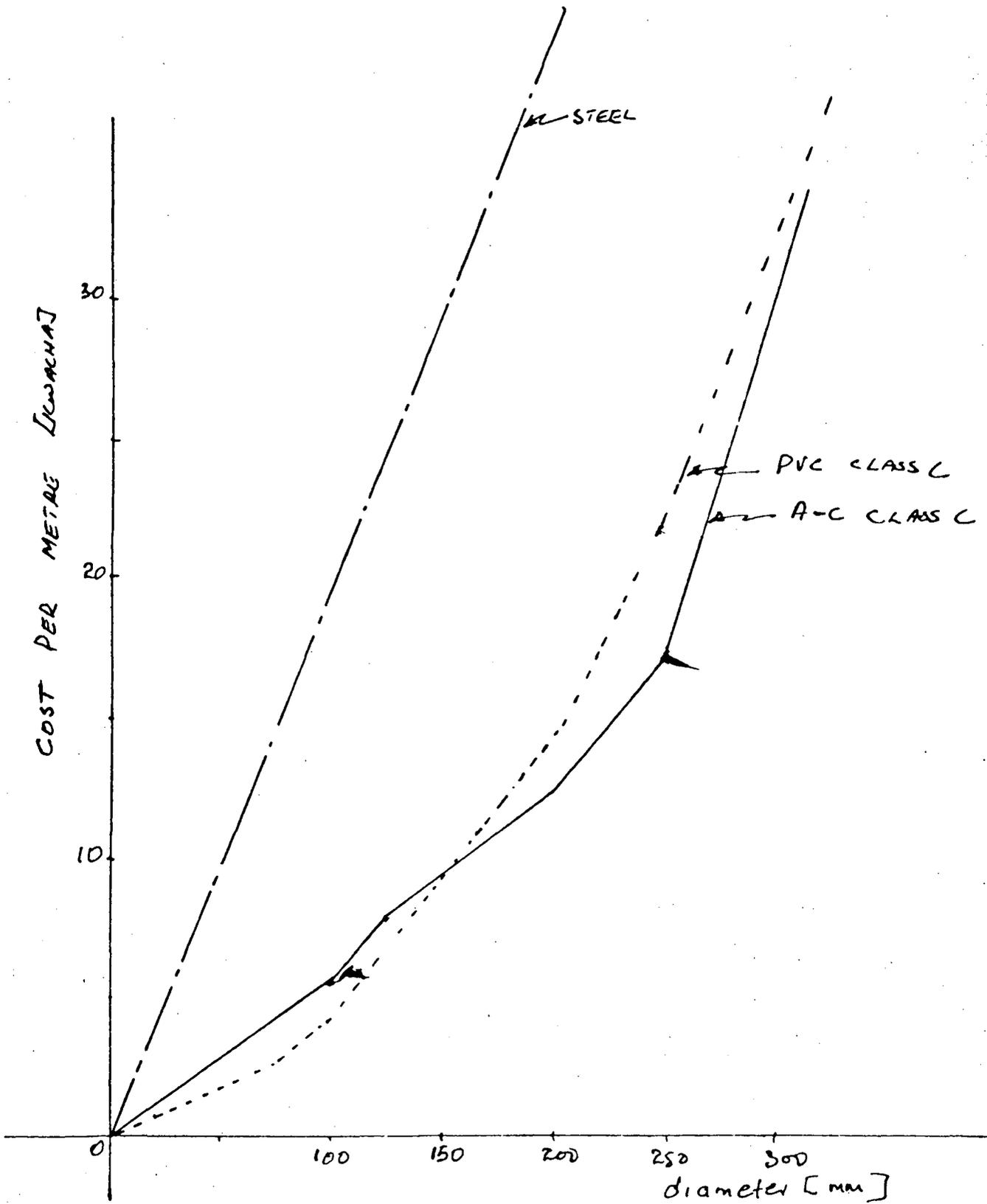
Fig. 15. Variation of costs with pipe diameter
