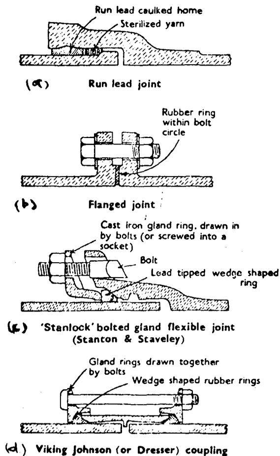
(a) Run-end-joint: Not so popular now but still in use. It requires high class workmanship. The lead which makes the grip has to be initially heated to  $400^{\circ}\text{C}$ . the joint is rigid.
