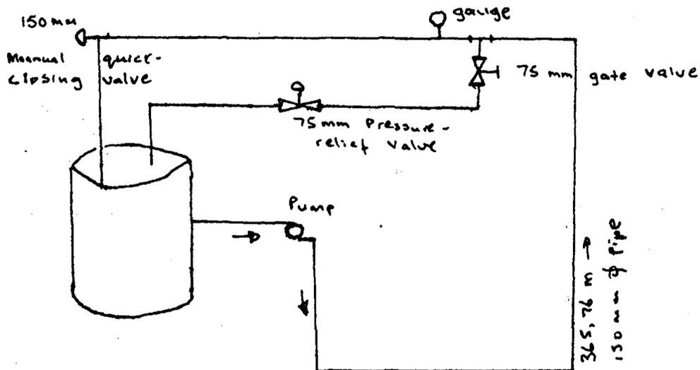
The 150 mm angle pattern valve fully closes in 6 seconds. At a flow rate of 45 l/s velocity in the 150 mm pipe is 1.98 m/s. The pumping pressure is 1930 N/m<sup>2</sup>. When the relief-valve is isolated from the system, surge pressures rise to between 1.79 and 1.82 x 10<sup>6</sup> N/m<sup>2</sup>. With the relief-valve in service surge pressure peak is between 4.8 and 5.5 x 10<sup>6</sup> N/m<sup>2</sup>. The response is not always as straight forward as that.
