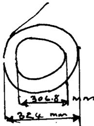
$$\begin{aligned} \text{Bursting Pressure} &= 0.588 \times 10^6 \text{ N/m}^2 \times 0.307 \text{ m} \times 1 \text{ m} \\ &= 0.1805 \times 10^6 \text{ N/unit length} \end{aligned}$$
