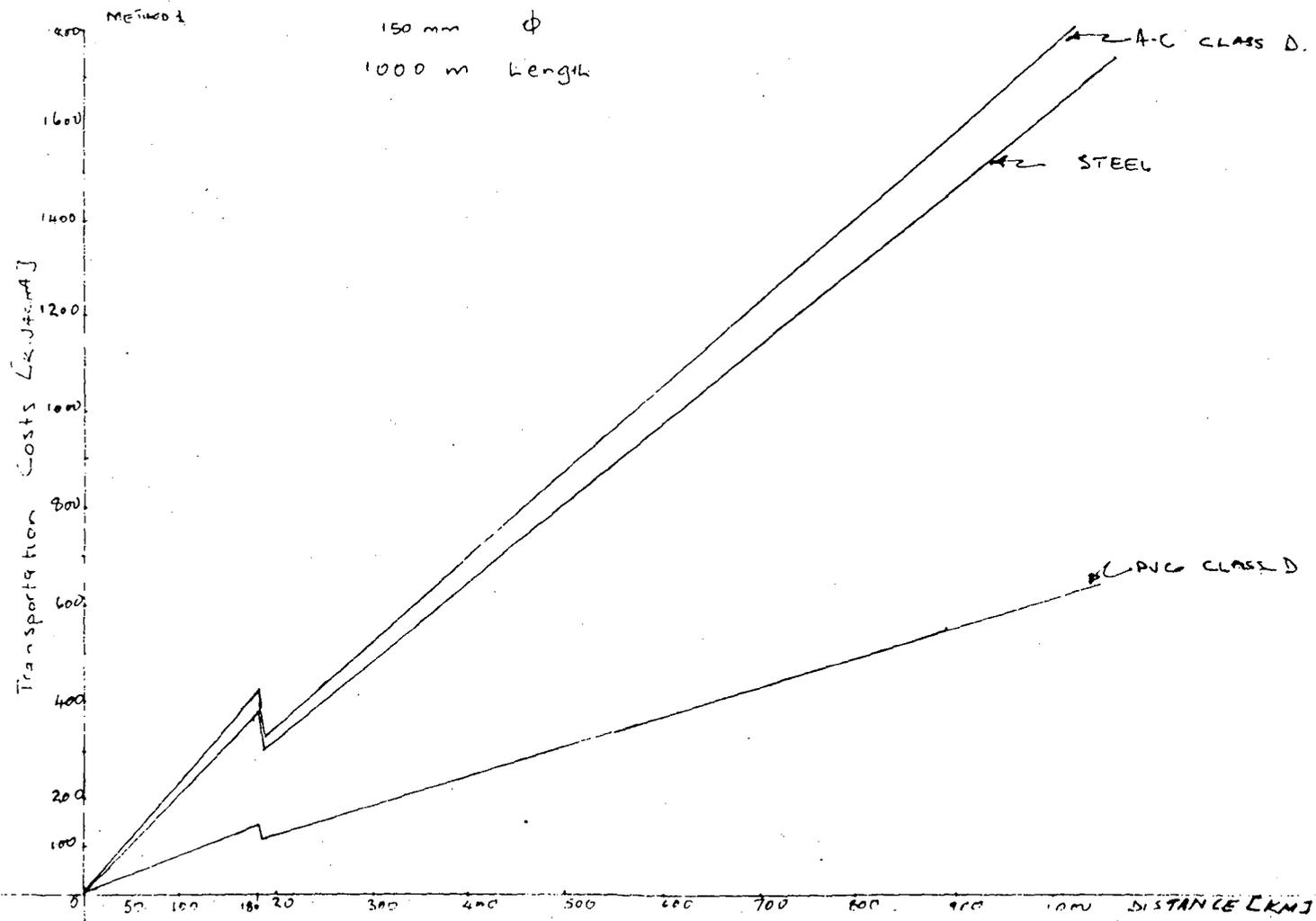
Fig. 16. Transportation costs vs distance (for charges per tonne pe km)
