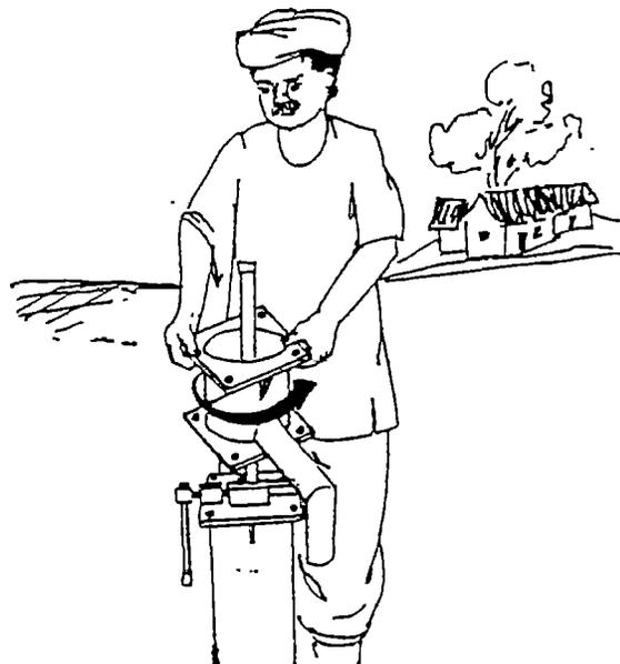
FIG:4.12 :REMOVE WATER TANK
