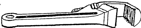
STILLSON PIPE WRENCH AT LEAST 3 SIZES, 610MM, 450MM, 350MM AND IF POSSIBLE 1000MM.
