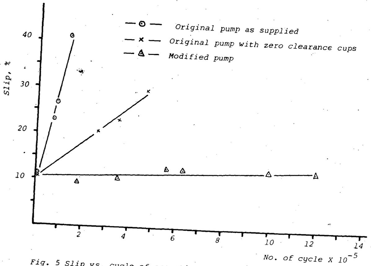
Fig. 5 Slip vs. cycle of operation.
