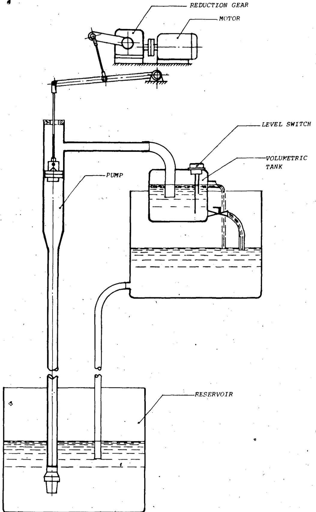
Fig. 2 A sketch of the test rig.
