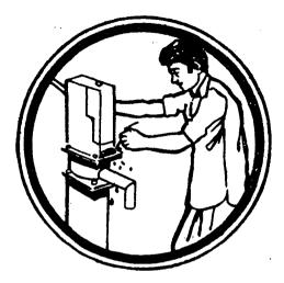
4. Open front cover. Clean out trash from drain-hole below this inspection cover.
