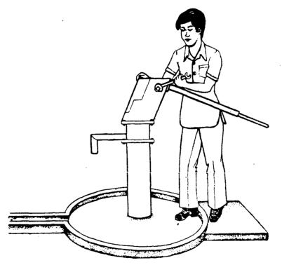
1. Are axle bolt and lock-nut tight?
