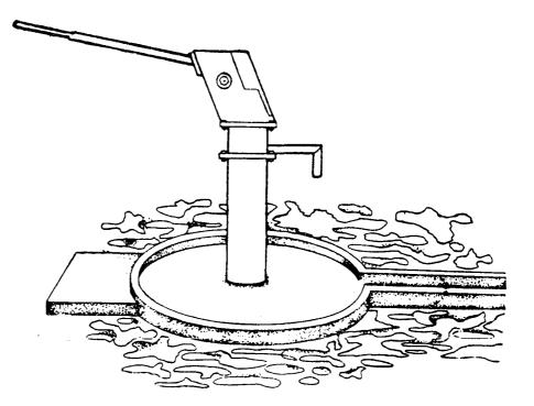
1. Excess water does not collect around the hand-pump .... Explain to the caretakers that excess water should not collect around the pump. It will make the surroundings unhygienic and unattractive, and stagnant water will become a breeding place for mosquitoes.
