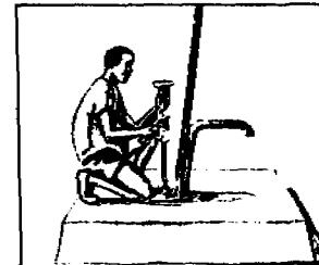
Immersed barrel with no mechanical part : no friction, therefore no wear, no corrosion.
