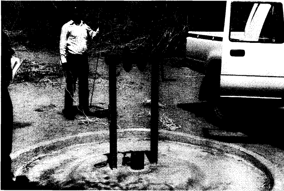
Figure 7: A forlorn, disused bucket pump.
