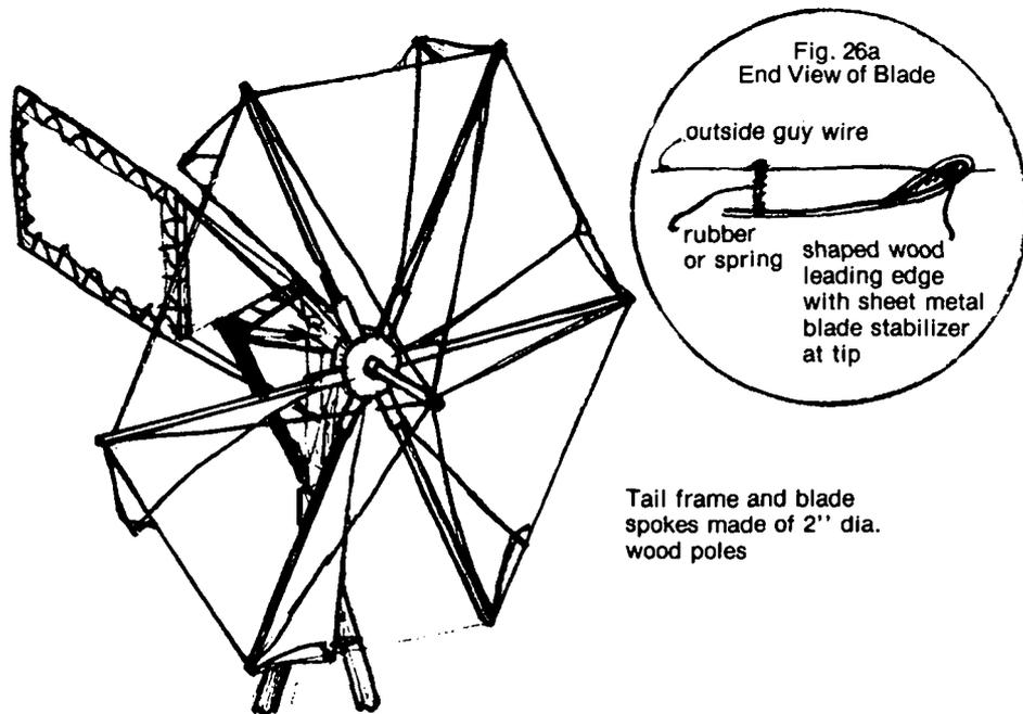
FIGURE 26. CLOTH OR HIDE BLADE AND TAIL CONSTRUCTION
