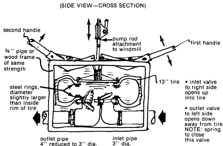
FIGURE 30. DIAPHRAGM PUMP FOR HIGH VOLUME, LOW LIFT IRRIGATION USES
