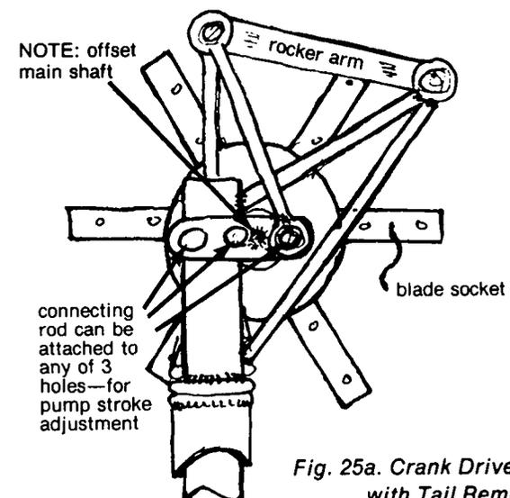
Fig. 25a. Crank Drive: Rear View with Tail Removed
