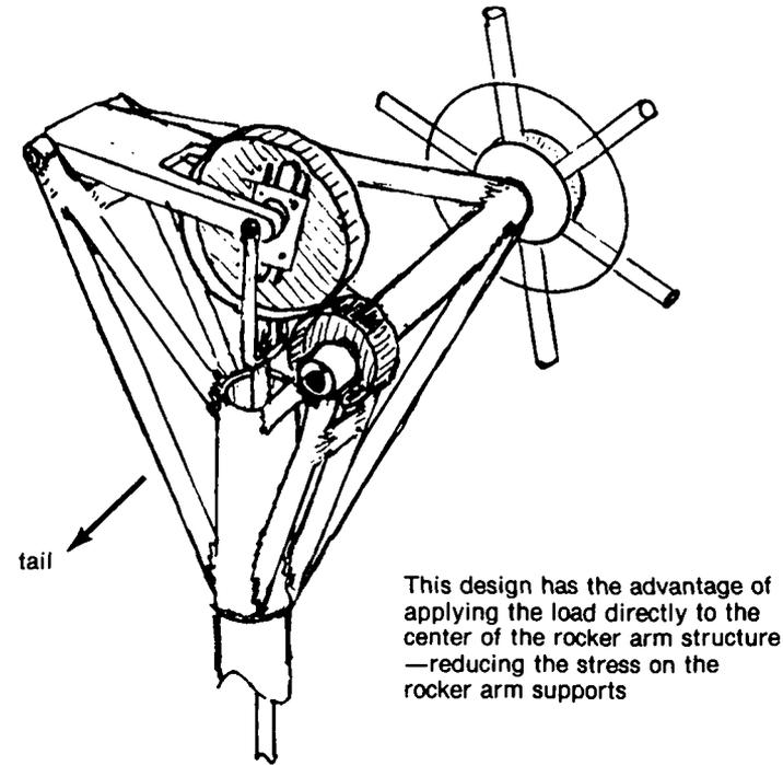
FIGURE 27. ALTERNATIVE ECCENTRIC WHEEL DESIGN
