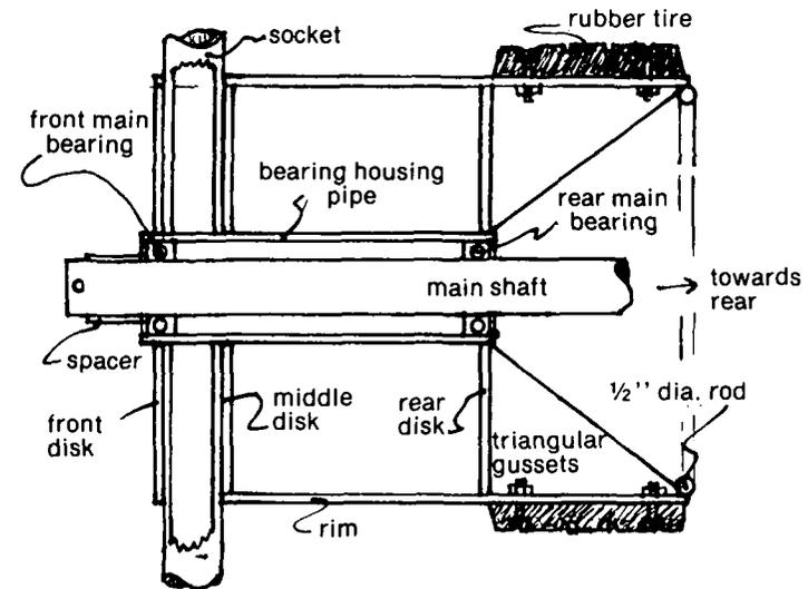
Fig. 15a. Hub Construction
