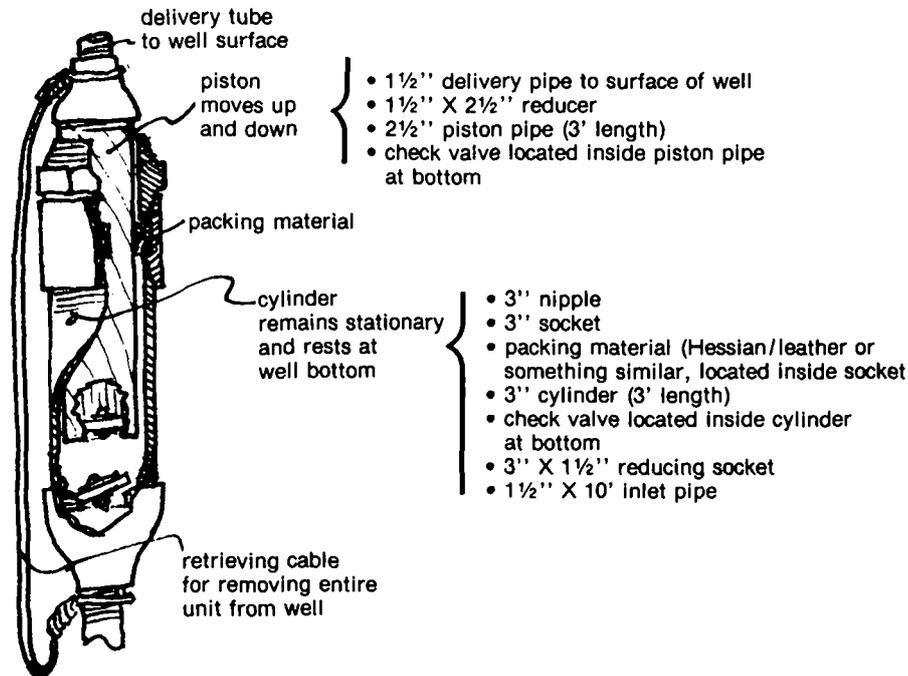
FIGURE 28. WORKING MECHANISM OF PISTON RAM PUMP
