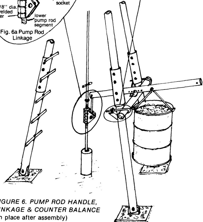
FIGURE 6. PUMP ROD HANDLE, LINKAGE & COUNTER BALANCE (in place after assembly)
