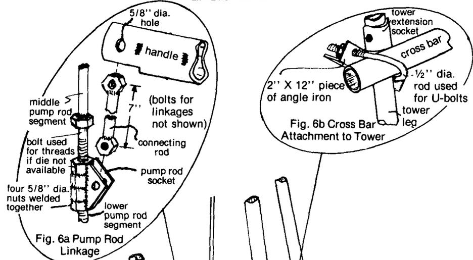
Fig. 6a Pump Rod Linkage
