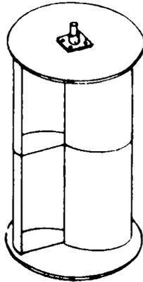
The Rotor has been designed in this form for moderate wind speeds and water-lifting up to 30 feet. Brace reports that a fair amount of "experimentation was needed to determine the best location of the pump relative to both the source and the discharge." Design of a simple diaphragm pump is also included.
