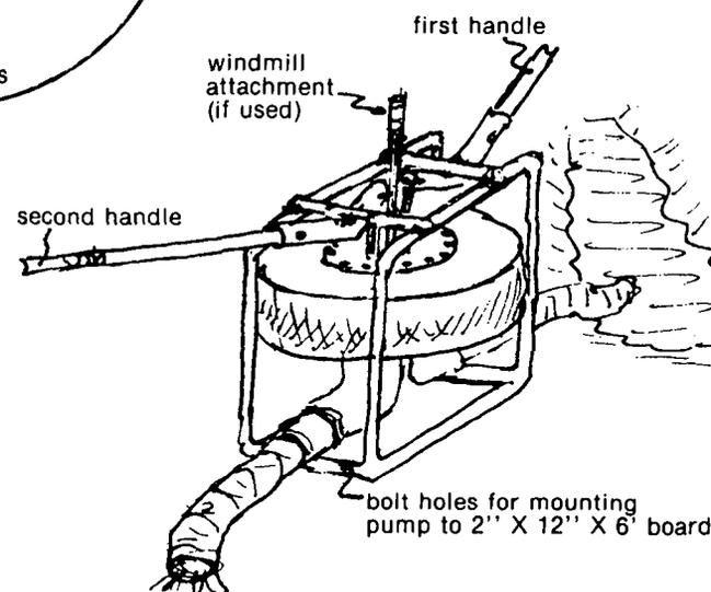
FIGURE 31. DIAPHRAGM PUMP IN ACTION
