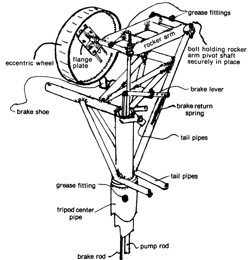
FIGURE 22a. ROCKER ARM, ECCENTRIC WHEEL, PUMP ROD, & BRAKE ROD IN PLACE (hub wheel not shown)
