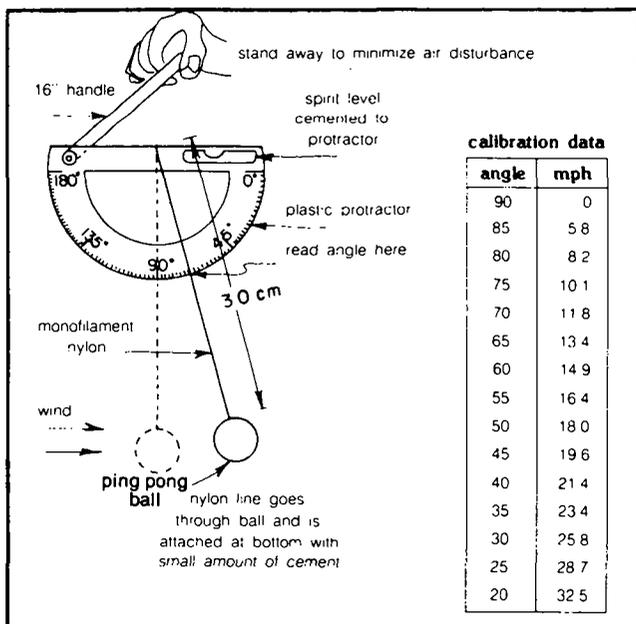
Figure 34. A Simple Hand-Held Wind Gauge with Calibration Data (based on C.L. Strong, *Scientific American*, October 1971).
