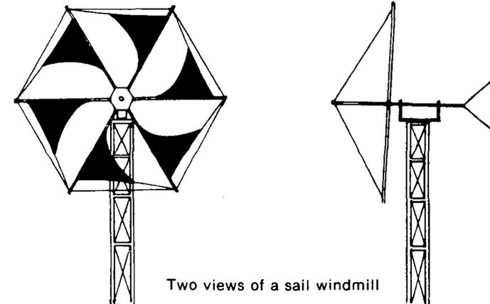
almost twice the rate of a commercial American Dempster multi-blade windmill. (This was partly because the sail windmill, due to its relatively light weight, was constructed so as to sweep a larger cross-sectional area. The sail windmill also outperformed 3 Savonius rotor windmills.) The most impressive design had the following characteristics: 16-foot diameter rotor when rigged with four sails, operating at a static head of 9 feet, would pump 1300 gallons of water per hour in a 14.5 mph wind.
