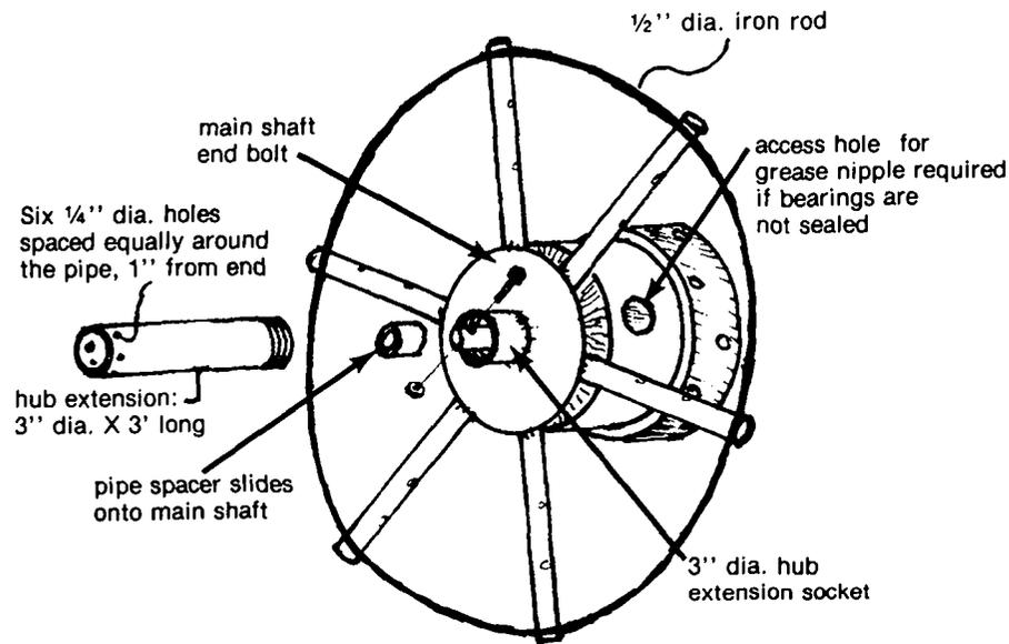
FIGURE 15. HUB WHEEL AFTER ASSEMBLY
