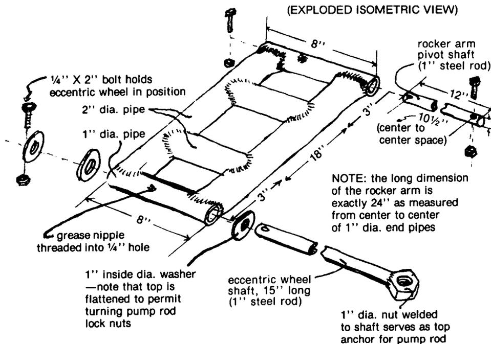
FIGURE 12. ROCKER ARM WITH PIVOT AND ECCENTRIC WHEEL SHAFT
