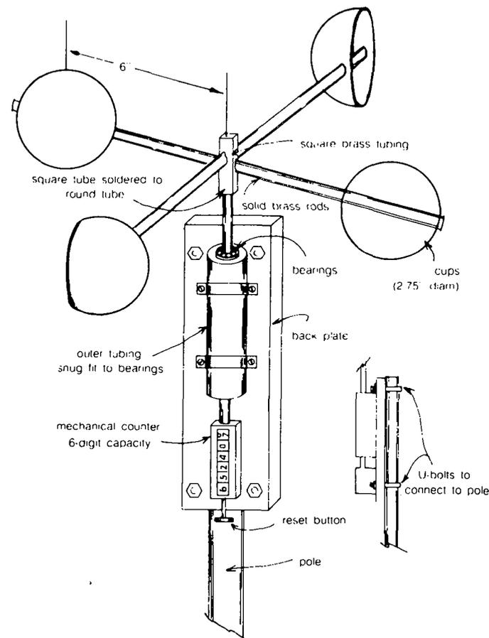
Figure 33. A Home-Built Cup Anemometer For Measuring Average Wind Speeds
