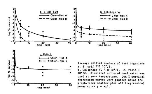
Fig. 1. Removal of microorganisms by two Chlor-floc tablets
