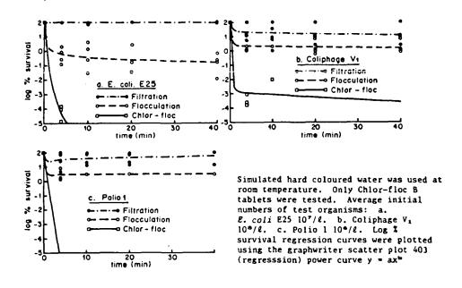
Fig. 2. Removal of microorganisms by filtration flocculation and a Chlor-floc tablet
