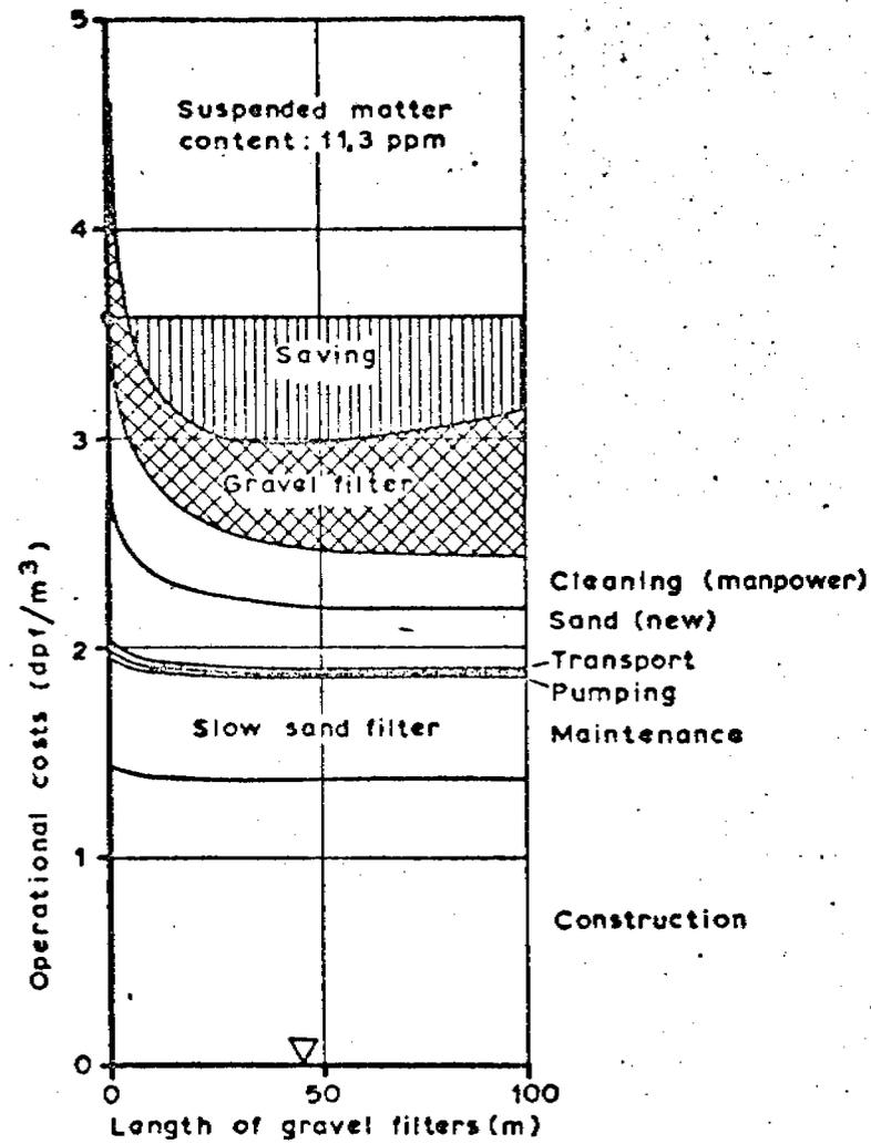
Fig 23 OPERATIONAL COSTS OF SLOW SAND FILTRATION WITH GRAVEL PREFILTERS
