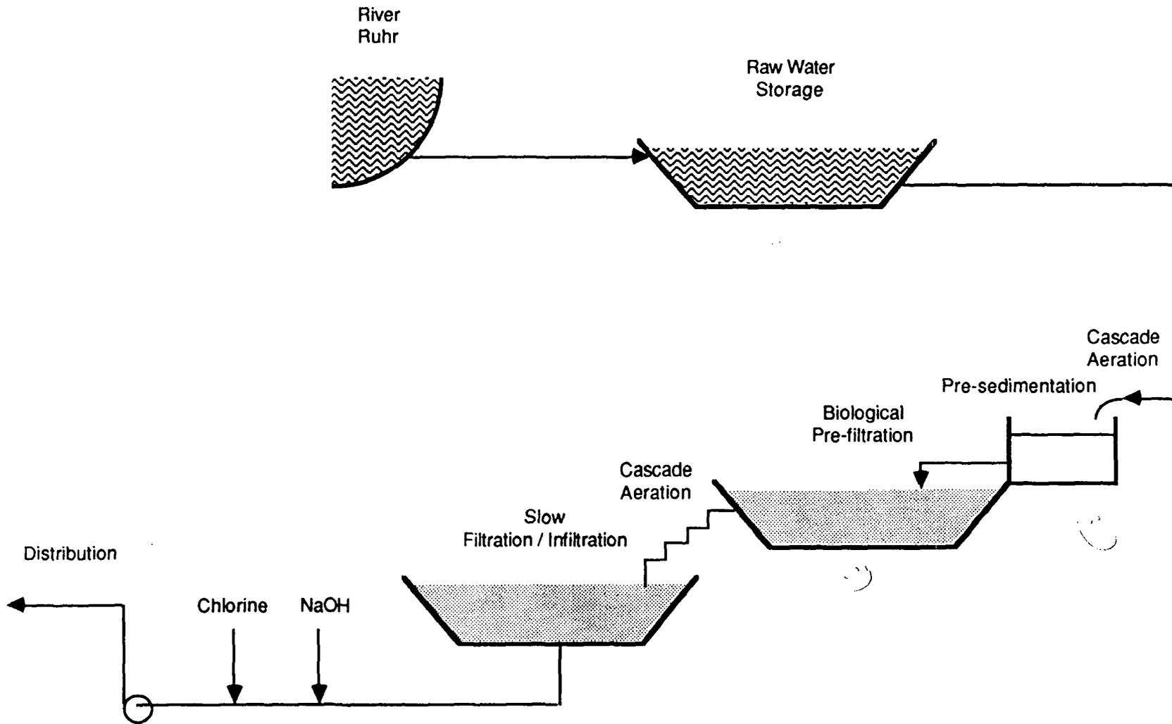
Figure 1. Process Schematic - Dortmund
