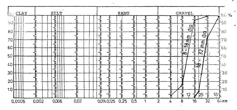
Figure 34. Grading of the coarse and fine gravel used in the horizontal filter during the investigation
