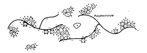
Figure 5. Agglomeration by specific adsorption and bridging
