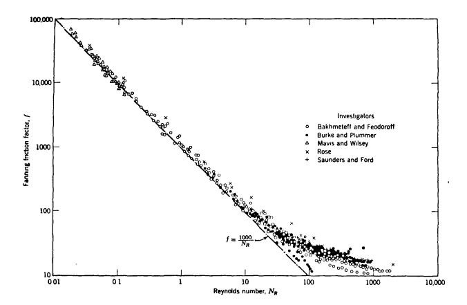
Figure 44. Relation of Fanning friction factor to Reynold's number for flow through granular porous media. Deviation from laminar flow occurs at Reynold's number = 10 (Todd, 1959)
