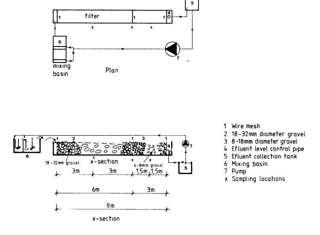
Figure 33. Schematic diagram for pilot filter layout and cross-section
