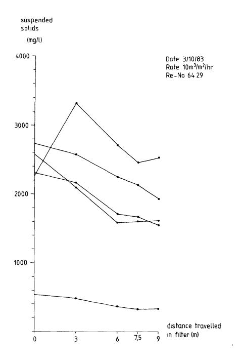
Figure 42. Pilot filter test. Suspended solids removal
