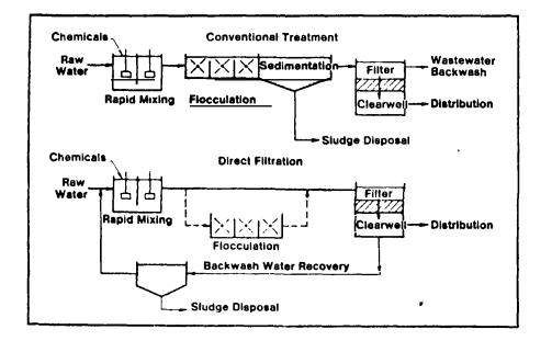
Figure 8. Comparison of conventional sedimentation filtration and direct filtration (Randtke, 1982)
