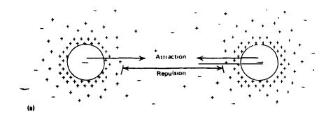
Figure 4 a. Electrokinetic répulsive and Van der Waal's attractive forces
