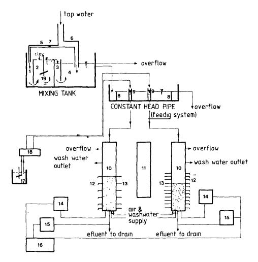
Figure 49. Schematic diagram of the experimental setup for direct filtration.
