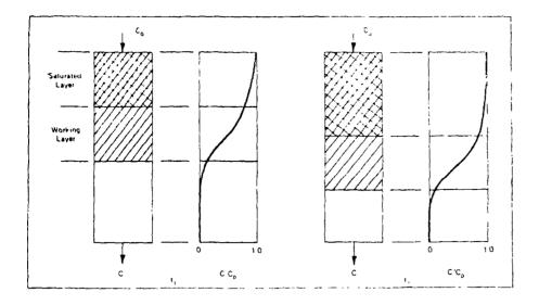
Figure 30. Progression of working layer through a filter (Adin and Rebhun, 1974)
