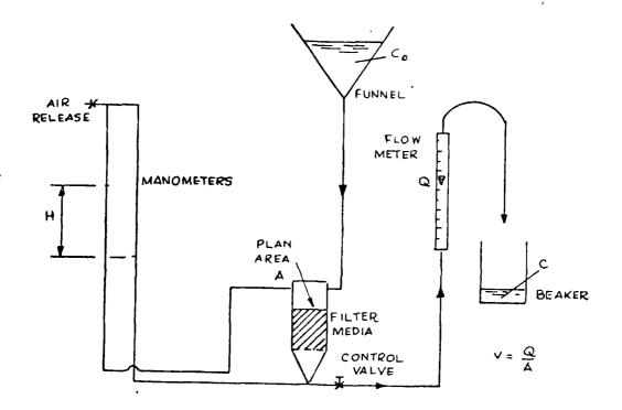
Figure 7. Diagram showing the principle of filterability apparatus (Ives, 1978)
