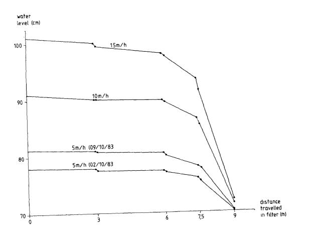
Figure 43. Piezometric readings for the various flow rates
