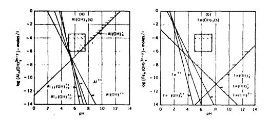
Figure 16. Equilibrium composition of solutions in contact with freshly precipitated  $Al(OH)_3$  and  $Fe(OH)_3$  (Stumm and O'Melia, 1968)
