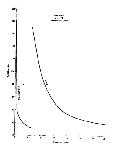
Figure 26. Comparison data of polyelectrolyte and alum dosages on turbidity removal (Beardsley, 1973)
