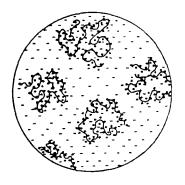
Figure 25. Possible arrangement of adsorbed polycations on a particle with low negative surface charge density (Bratby, 1980)
