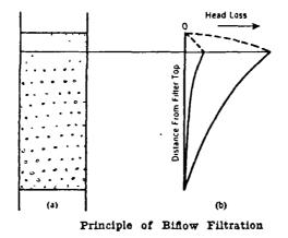
About 20 per cent of the filtrate enters from the top of the column The other 80 per cent enters from the bottom. The sand at the top is fine, that at the bottom, coarse. The line running from 11(a) to 17(b) represents the point at which the filtrates coming from opposite directions meet. In 11 (b), the left-hand curves show initial head loss The right-hand lines show the loss after some time of operation.
