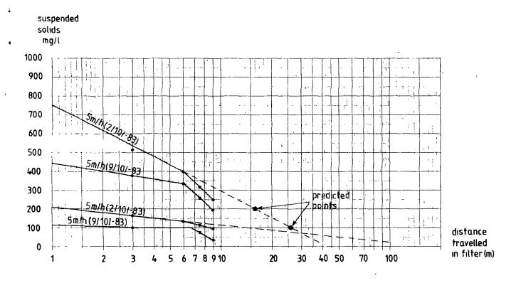
Figure 47. Prediction of filter length
