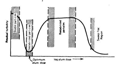
Figure 18. Alum dose versus residual turbidity for water coagulation/flocculation. The residual turbidity is that which remains in a test solution to which alum was added. After mixing to simulate that which occurs in a water treatment plant, the sample is allowed to settle for 30 min before turbidity is measured.
