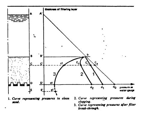
Figure 12. Distribution of pressure in monograded filter layer (Degrémont, 1979)
