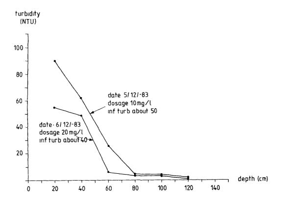
Figure 60. Effect of depth on turbidity removal
