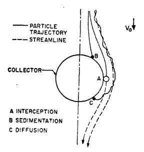
Figure 1. Basic transport mechanisms in water filtration (Yao et al, 1971)
