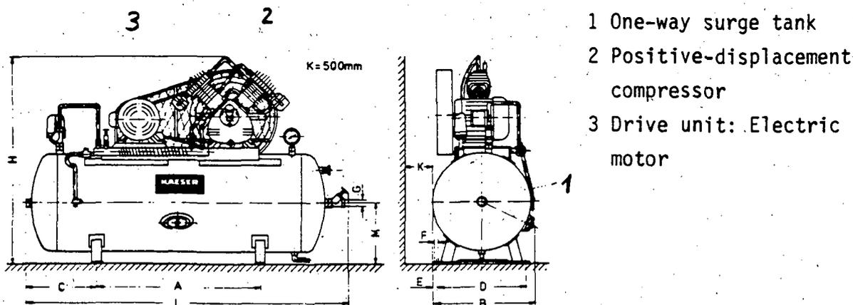
Fig. 4: Compact compressor unit
