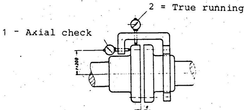
Fig. 1: Realignment of couplings
