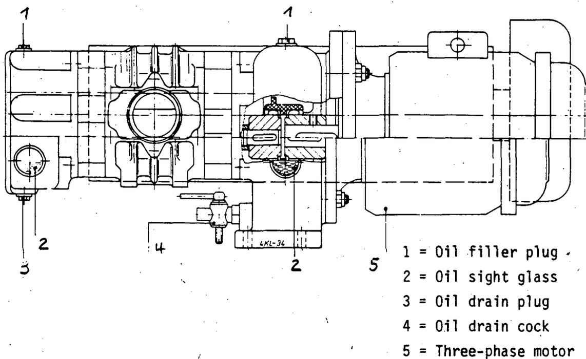
Fig. 3: Oil filler points and sight glasses on a rotary blower
