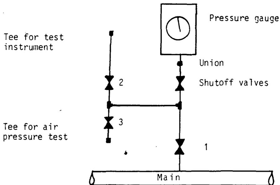
Fig. 4 - Piping arrangement for pressure gauge field testing.
