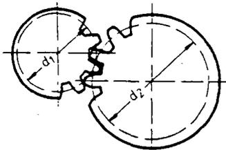
Since the gear wheels intermesh, they must rotate with the same circumferential velocity.
