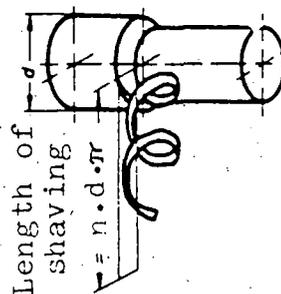
If the "n" revolutions are completed in a specific time, e.g. per minute, there results a rotational speed.
