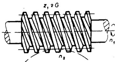
If a single-threaded worm is turned once, the worm wheel moves forward by one tooth.
