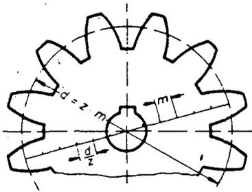
The module was introduced as a dimension to represent these equivalent ratios. The module is given in mm. Module 1 is equivalent to a pitch of 3.14159.... mm ( $\pi$ ), measured along the pitch circle. For measurements along the radius, however, module 1 = 1 mm.
