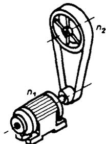
This is the ratio of the speed of the driving wheel to that of the driven wheel.
