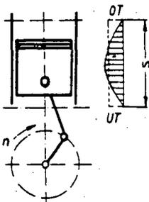
$$v_m = 2 \times s \times n \left[ \frac{\text{m}}{\text{min}} \right]$$
