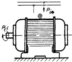
$$\text{Efficiency} = \frac{\text{work output}}{\text{work input}} = \frac{\text{useful work}}{\text{effort}}$$
