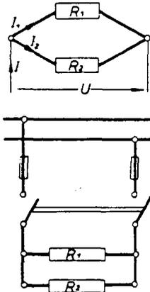
The same voltage  $V$  is applied to all resistors placed side by side with their corresponding ends joined together.
