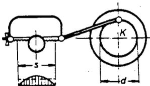
At 1 revolution from point K, the distance is  $2 \times s$ , at "n" revolutions from point K, the distance is  $2 \times s \times n$ . At n revolutions per min,
