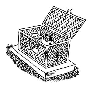
The place where your Water Point is connected to the branch pipeline is called a Water Point offtake. At the offtake there is a valve so that you can stop the water going to your Water Point if you need to. There is also a water meter which measures how much water has gone to your Water Point. Each Community pays according to how much water has been used at their own Water Point. The valve and the water meter are inside metal cages to stop them from being damaged.
