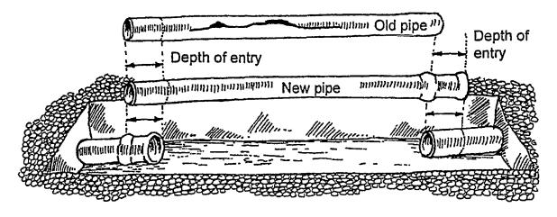
6. Use a file to make new spigot ends on the new piece of pipe and the pipe in the trench.
