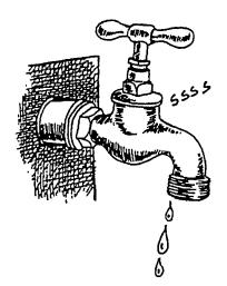
This problem happens when the tap washer can not make a watertight seal against the seat. Replace the tap washer and clean the seat. If this does not work then either the seat is damaged or the spindle is worn out and you must replace the tap.
