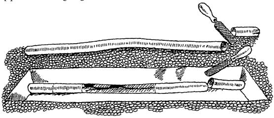
Clean both pipe ends and one of the connectors thoroughly with a soft clean cloth and some clean water. When making the connection make sure that both pipes are pushed firmly into the connector. The connector should be tightened firmly by hand, you do not need to use the pipe wrench.
