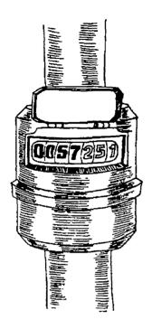
There are many different types of water meter. Two of the types are shown here. There is a plastic cover which can be opened to see a small window. Inside the window are the numbers which give you the water meter reading.
