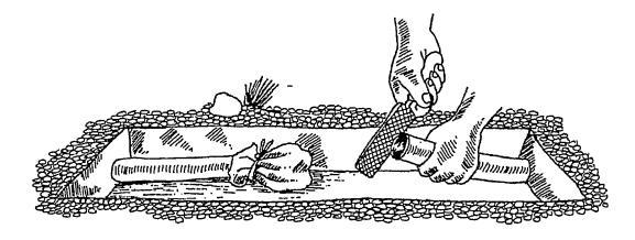
7. Before you try to put the new piece of pipe in place, you may have to extend the trench so that there is flexibility alone, the length of the pipeline. You need some flexibility to be able to get the final spigot into the socket
