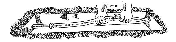
8. Make one joint at a time. Before pushing the spigots and sockets together, make sure they are absolutely clean. Apply jointing oil to the outside of the spigots and to the inside of the sockets. If you do not use oil the pipes will be difficult to push together and the rubber seal can be damaged.
