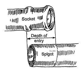
The full name for PVC is Poly Vinyl Chloride. This kind of pipe comes in straight sections six metres in length. Every pipe has a socket at one end, the other end is called the spigot. It is not very flexible so a bend must be fitted into the pipeline if you want it to change direction. PVC pipe for clean water is blue and common diameters are from 25 mm to 250 mm. PVC pipes lose their strength if they are left out in the sun and so any spare pipes which you keep must be covered.
