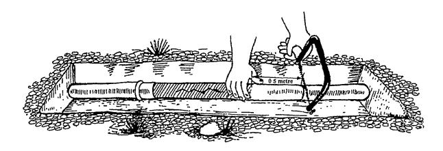
4. Carefully pull the damaged piece of pipe out of the socket. It is very important to make sure that no dirt or sand gets into the socket otherwise it will never make a good joint again. Tie the other plastic bag, over the open end of the pipe.
