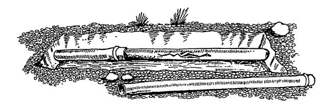
3. Cut the pipe with a hacksaw. Make the cut half a metre from the damaged part of the pipe. Be sure to cut the pipe exactly square with its length. Tie one of the plastic bags over the open end of the pipeline so that no dirt can get into it.
