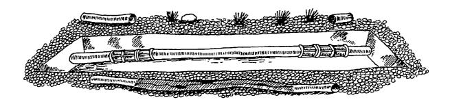
5. The repair must now be tested to make sure that it was successful. Turn the water supply to the pipe back on again. Inspect the new pipe and connections to see whether there are any leaks. Leave the hole open for a few hours to be absolutely sure.
