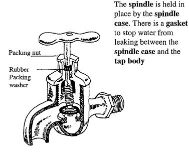
Water does not pass up the side of the spindle because it is stopped by a rubber packing washer. The rubber packing washer is held in place by the packing nut (sometimes called the gland nut)
