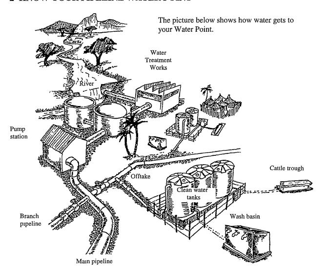
The water which comes out of your pipeline Water Point starts off in a river or a borehole. The water is taken from the river and goes to the Water Treatment Works. At the Water Treatment Works the water is cleaned so that it is safe to drink. There are large tanks for storing a reserve of clean water at the Water Treatment Works.
