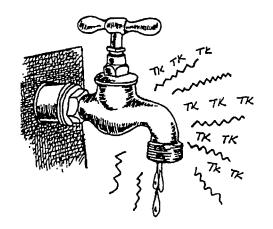
Taps make a loud noise when the tap washer is not held firmly on the spindle. Tighten the nut holding the washer onto the spindle. If you can not tighten this nut then you must replace the tap before it breaks down completely.
