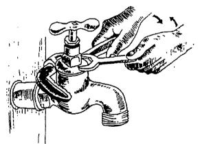
3. Unscrew the nut from the end of the spindle and remove the metal washer. You can now remove the rubber tap washer and replace it with a new one. Replace the metal washer and tighten the nut firmly.
