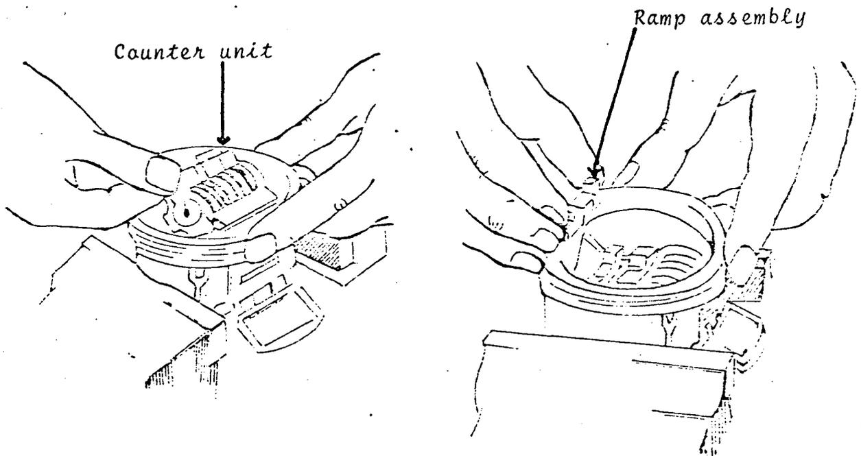
FITTING AND LOCKING COUNTER UNIT IN POSITION
