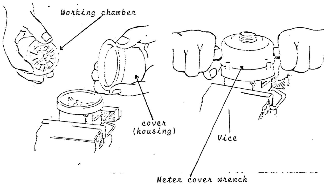
REPLACING WORKING CHAMBER AND SCREWING ON CHAMBER HOUSING
