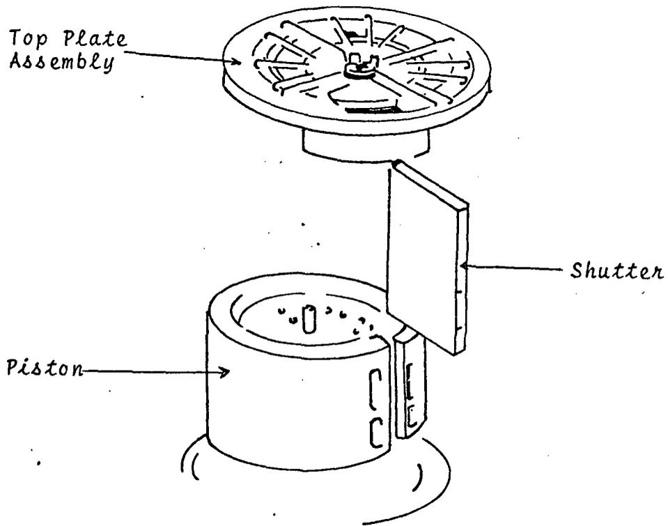
REMOVING TOP PLATE ASSEMBLY
