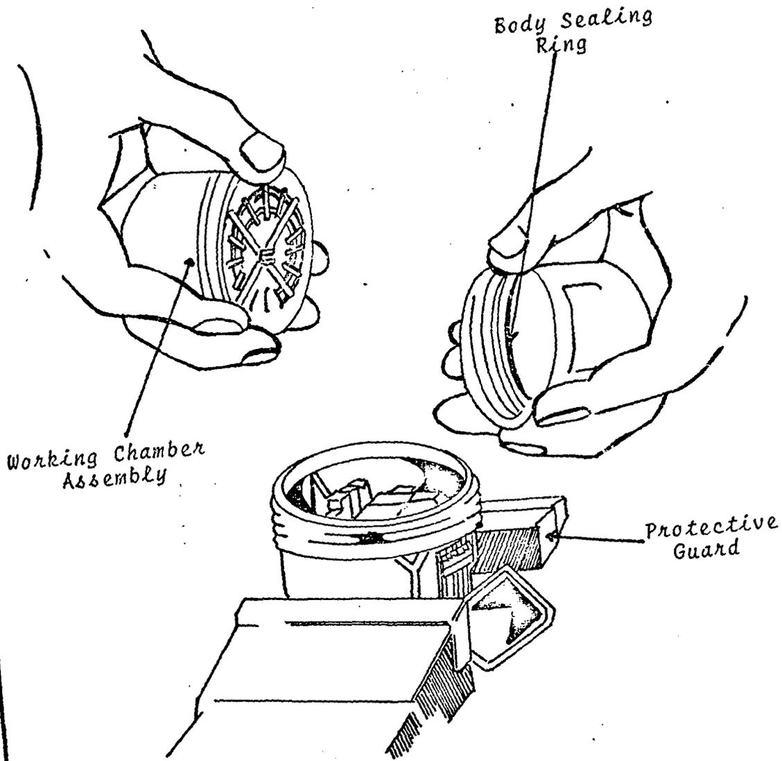
LIFTING OUT WORKING CHAMBER ASSEMBLY
