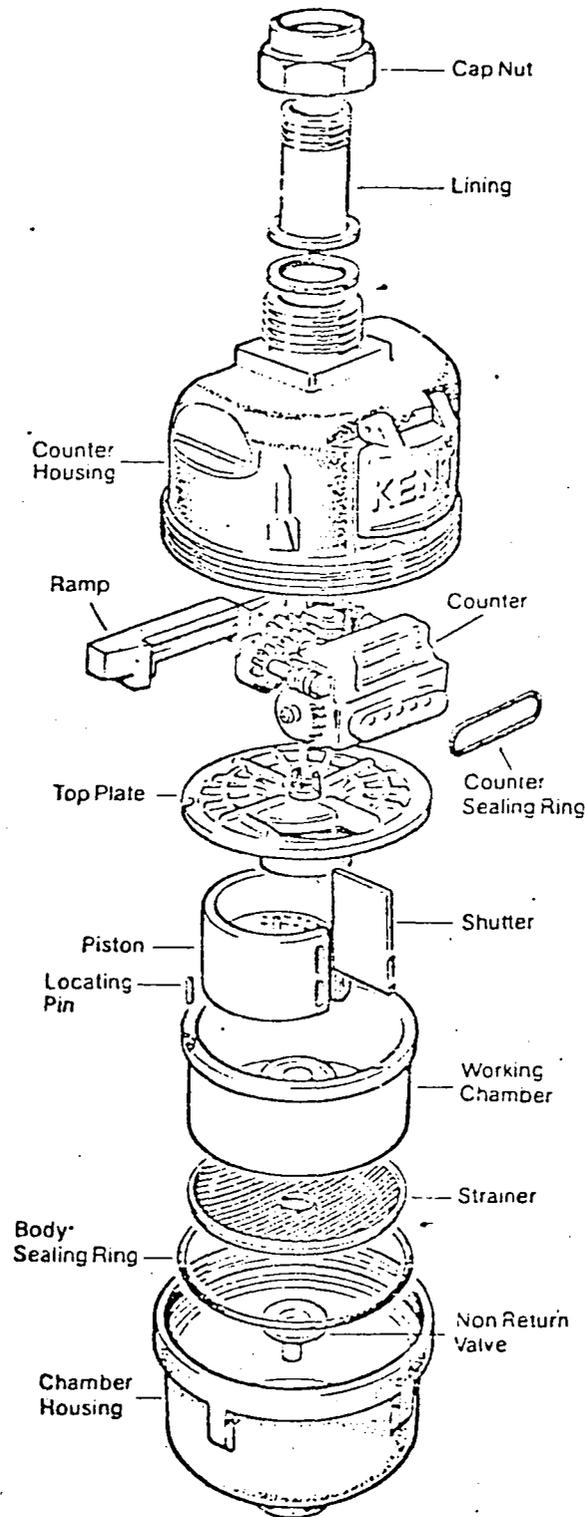
INTERNAL AND EXTERNAL PARTS OF A KENT WATER METER
