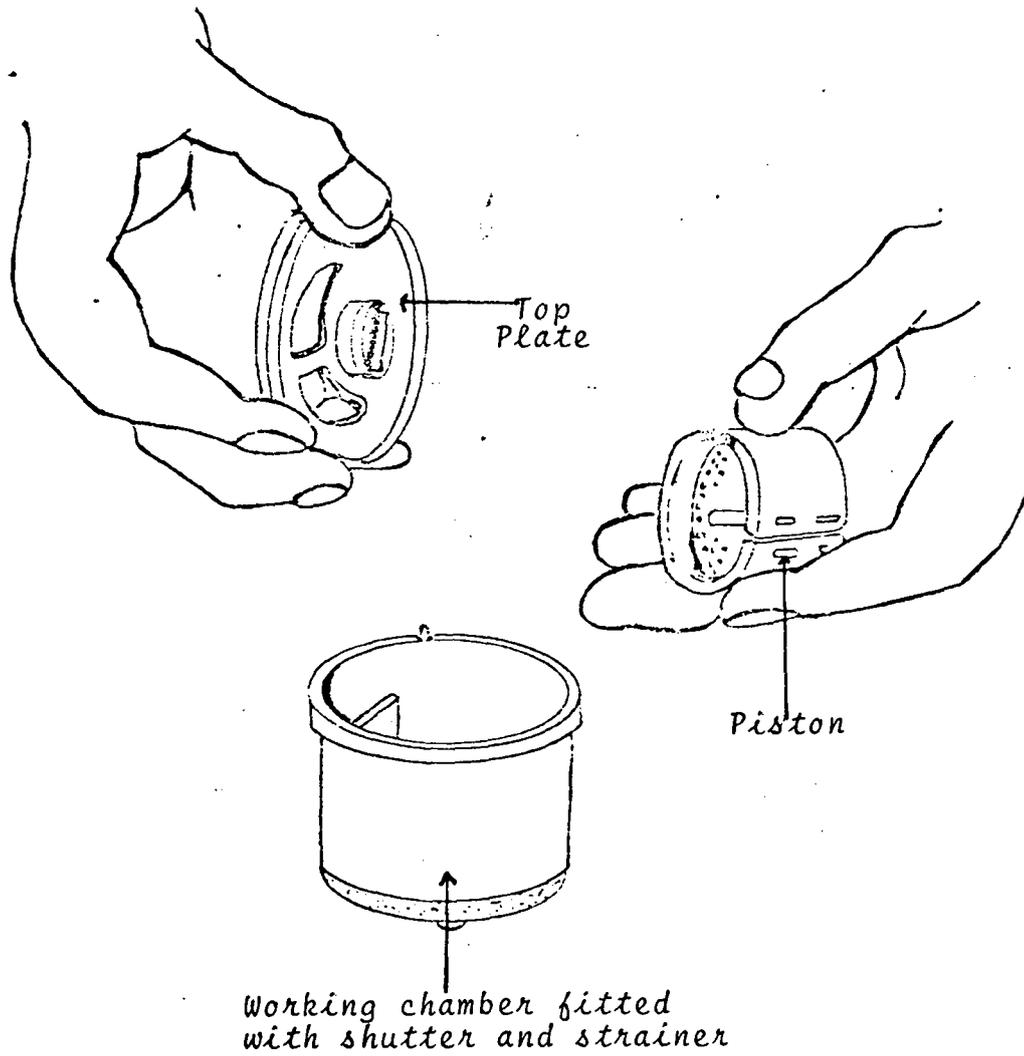
INSERTING THE PISTON AND REPLACING THE TOP PLATE WITH CHAMBER
