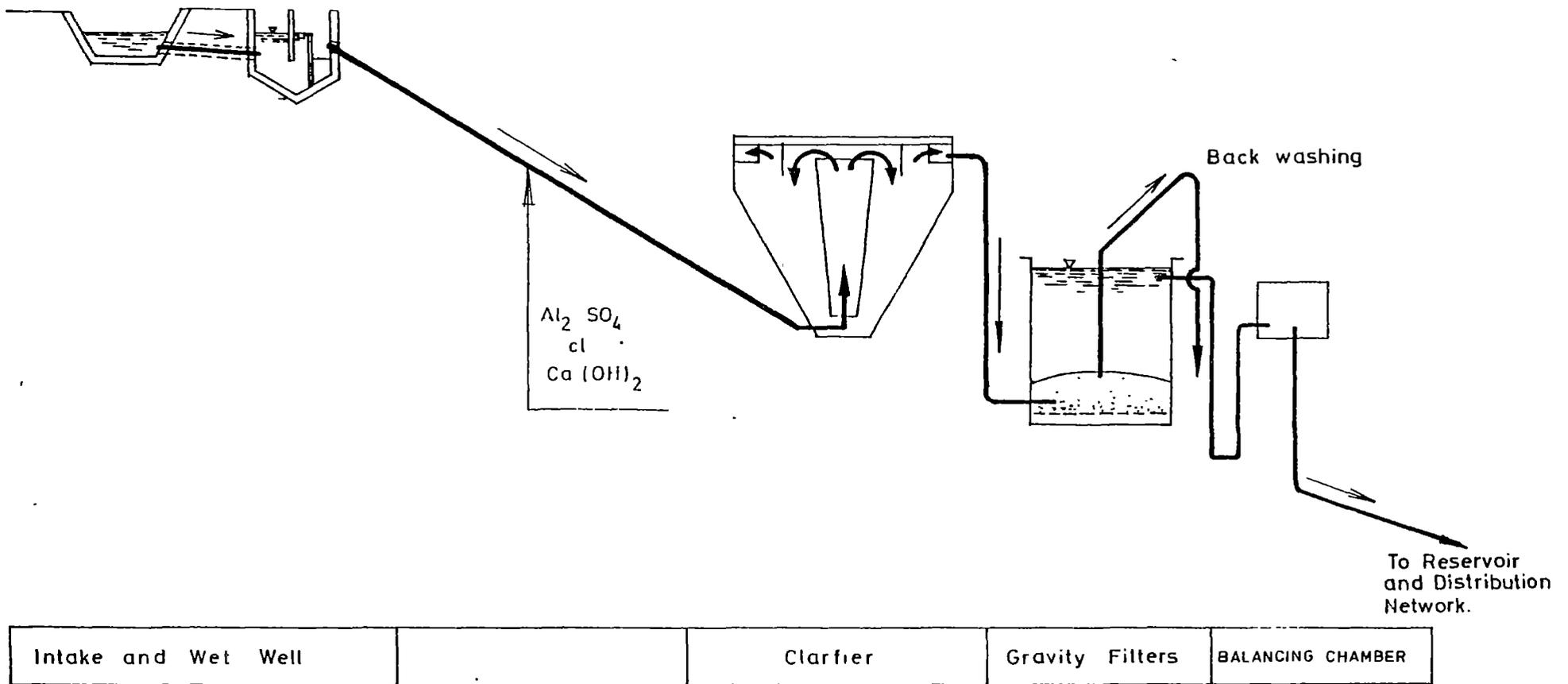
Figure 7. Schematic view of the treatment plant in Awassa (GWE, 1978).
