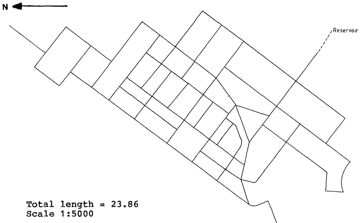
Figure 11. Layout for the distribution network of Awassa town water supply system (GWE, 1978).
