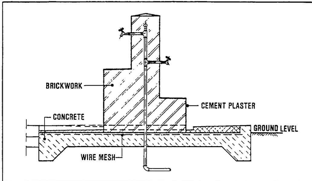
Figure 2. Cross section of a multiple tap standpipe (Hofkes, 1985)
