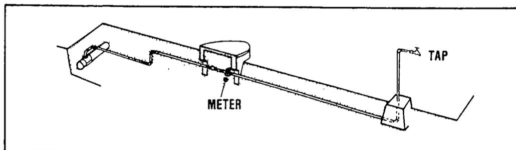
Figure 1. A typical yard connection (Hofkes, 1985).
