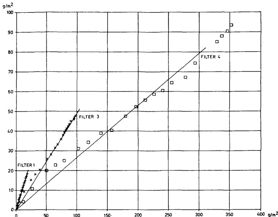
Fig. 5. Column experiments 1975/76. Sorbed phosphorus as a function of the phosphorus supply, filter 1, 3 and 4.
