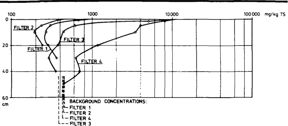
Fig. 4. Column experiments 1975/76. Contents of COD in soil samples, filter 1—4.
