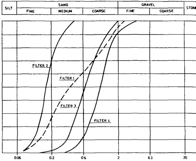
Fig. 2. Column experiments 1975/76. Texture, filter 1—4.
