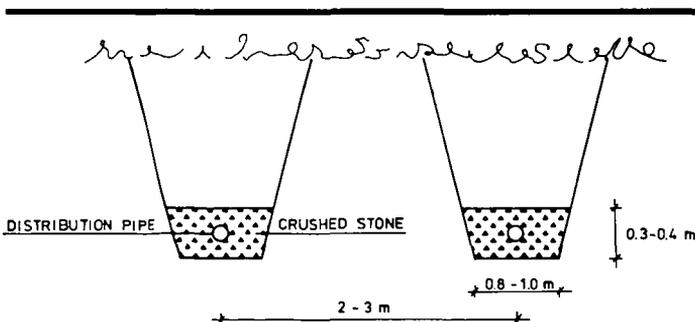
Fig. 7. *Disposal trenches. Section.*
