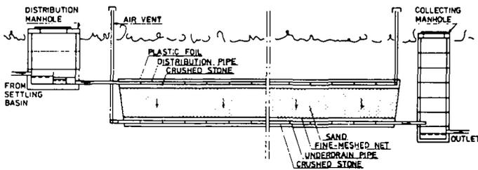
Fig. 1. Subsurface sand-filter. Section.
