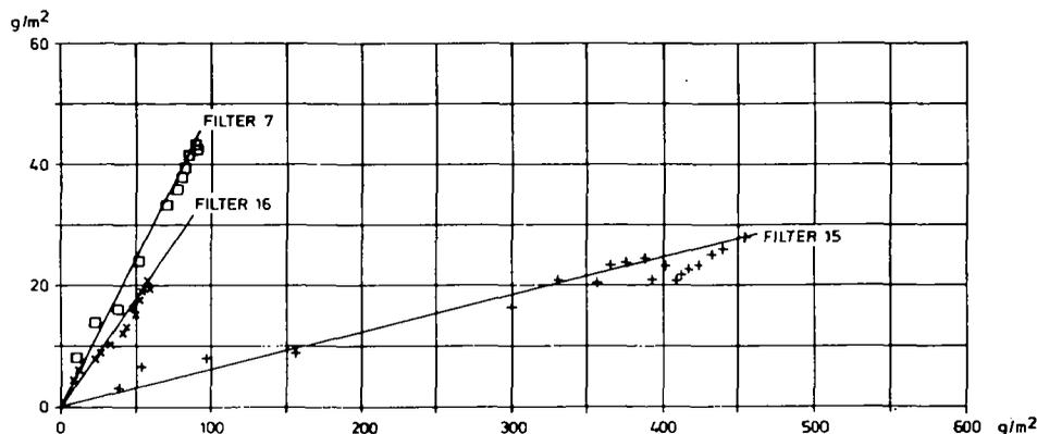
Fig. 6. Column experiments 1976/77. Sorbed phosphorus as a function of the phosphorus supply, filter 7, 15 and 16.
