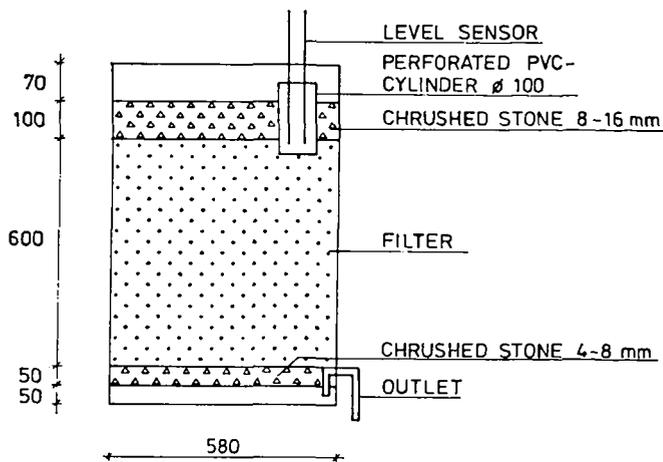
Fig. 1. Column construction.
