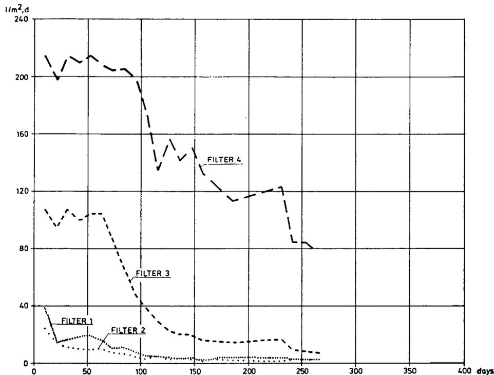
Fig. 3. Column experiments 1975/76. Hydraulic load, filter 1—4.
