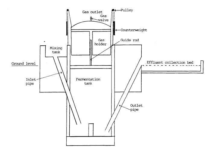
Figure 2. A Typical Indian Biogas Plant
