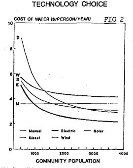
Water Use 20 lpcd Pumping Lift 20 meters
