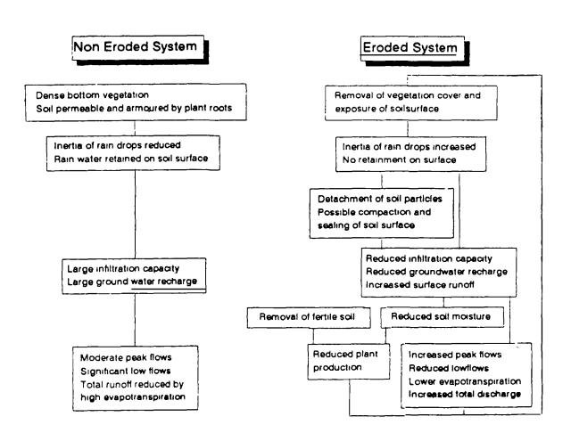
Figure 2.14. - Hydrological processes in eroded and non-eroded soil systems
