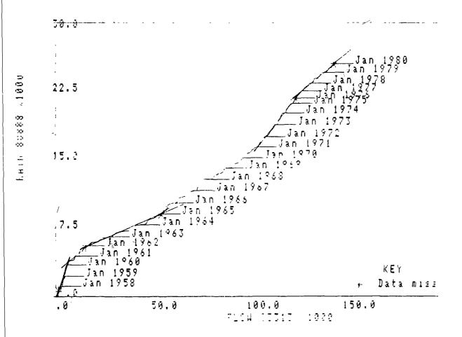
Figure 5.2 Double mass curve, River Kafu flow versus rainfall
