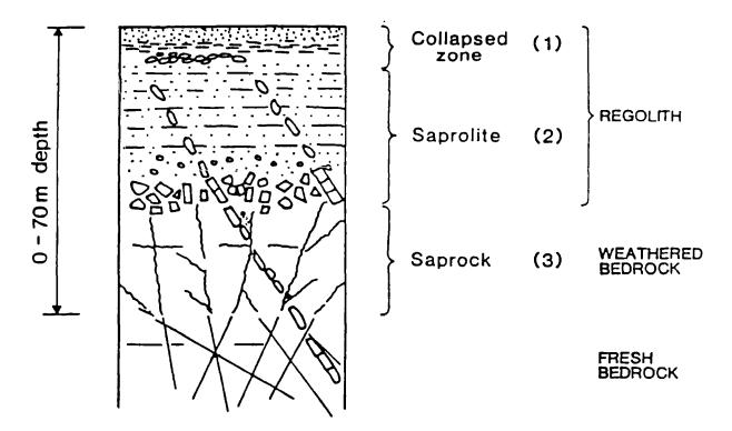
Figure 4.2 - Typical in-situ weathered regolith profile and underlying crystalline bedrock
