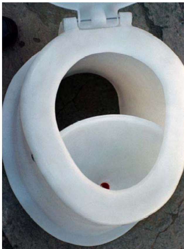
Figure 2: A urine diversion pedestal made from rotationally moulded plastic, installed in the village of Sinyondweni near Umtata, Eastern Cape. Urine is collected in the front compartment and led away by a pipe. Faeces drop through the rear opening and are collected in a receptacle beneath.
