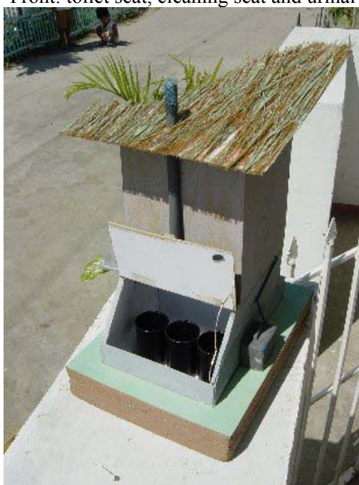
Back: processing chamber with collection buckets
