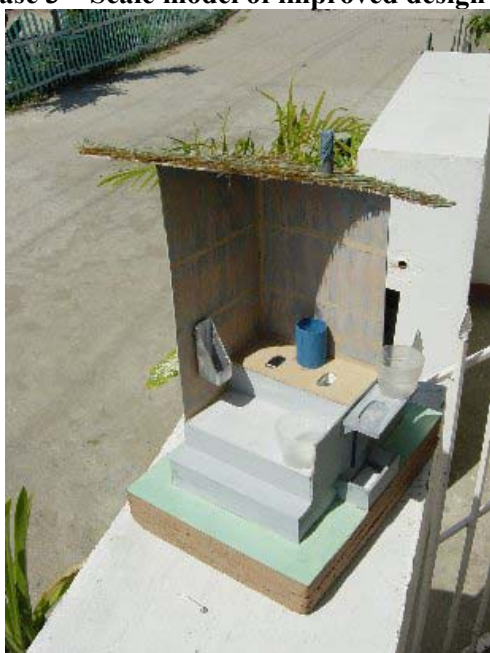
Front: toilet seat, cleaning seat and urinal
