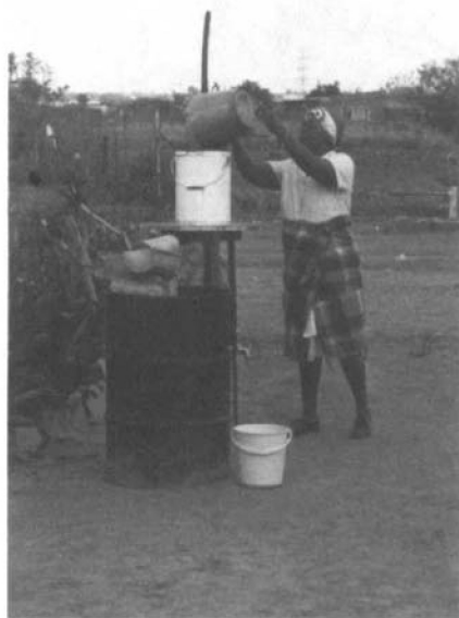
Using the iron removal plant: note tubewell behind to the right.
