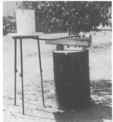
A completed iron removal unit in a homestead yard.
