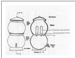
Figure 1. Setup of the filtration system with candle stick
