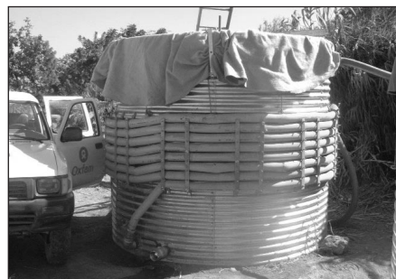
Oxfam's Field Upflow Clarifier, tested in Gonaives
