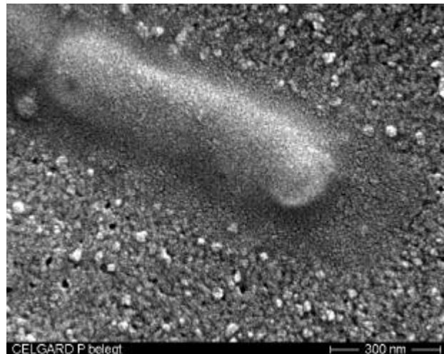
Figure 2: Electron-microscopic enlargement showing the surface of a membrane with captured particle (bacterium?)
