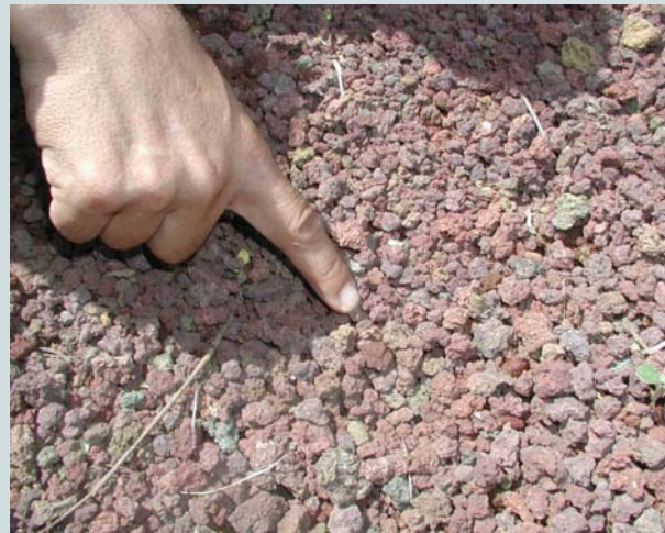
The volcanic filter material ( hormigón rojo ) used for constructed wetlands in Central America. Source: Martin Gauss, 2006.
