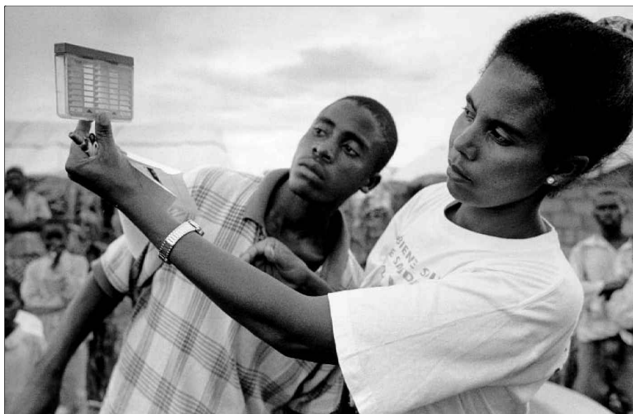
Using a chlorine comparator to measure residual chlorine content Photo credit: Crispin Hughes
