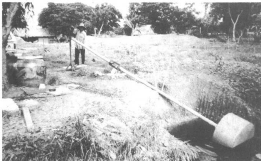
A watertight cylindrical drum supports the coil.
