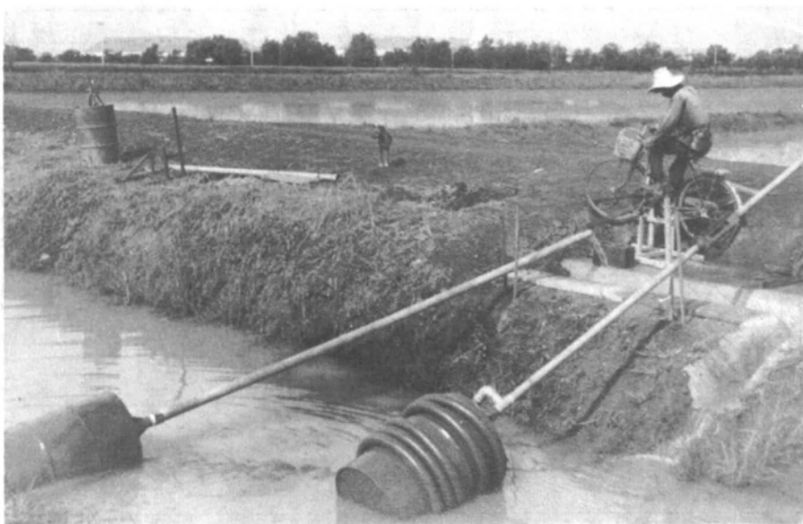
Pedal power provides ample energy to run the pump.
