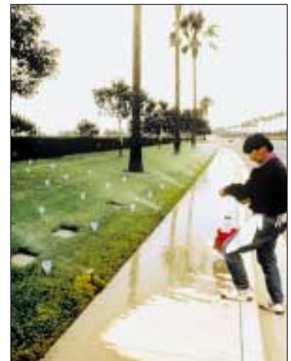
Every irrigation station received a detailed analysis including flow testing, precipitation rate, pressure and uniformity. The photo shows an irrigation station being measured with a "can test."
