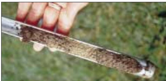
An example of a core-extracting soil probe.
