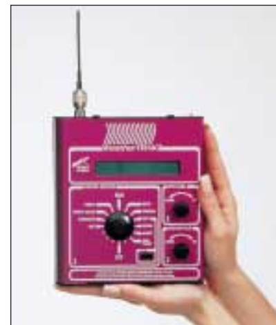
Above: The new wireless technology transmits local weather-station data each week directly to homes equipped with ET-receiving irrigation controllers. Right: The ET-signal irrigation controllers.
