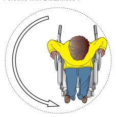
Figure 1. A turning circle for wheelchairs<sup>5</sup>
