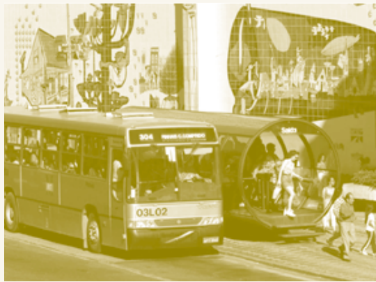
CURITIBA'S ECO-EFFICIENT, BUS-ONLY TRANSPORTATION SYSTEM IS A MODEL FOR CITIES AROUND THE WORLD. THE "SPEEDY BUS" RUNS ALONG A DIRECT LINE AND STOPS ONLY AT TUBULAR STATIONS SPECIALLY DESIGNED TO MOVE PASSENGERS QUICKLY.
