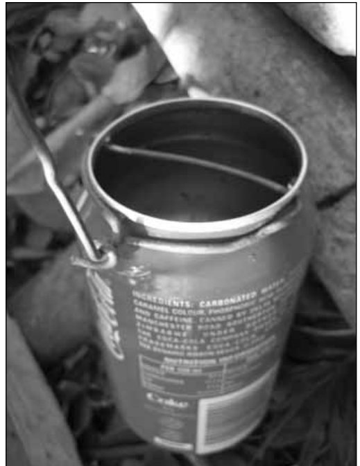
Wire is cut and passed through the two upper holes and twisted to form a handle with a hook on the end
