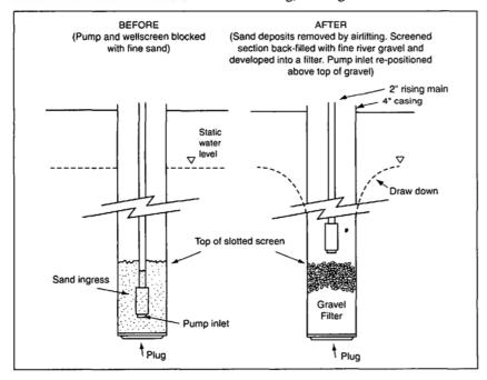
Figure 1. Borehole rehabilitation schematic.
